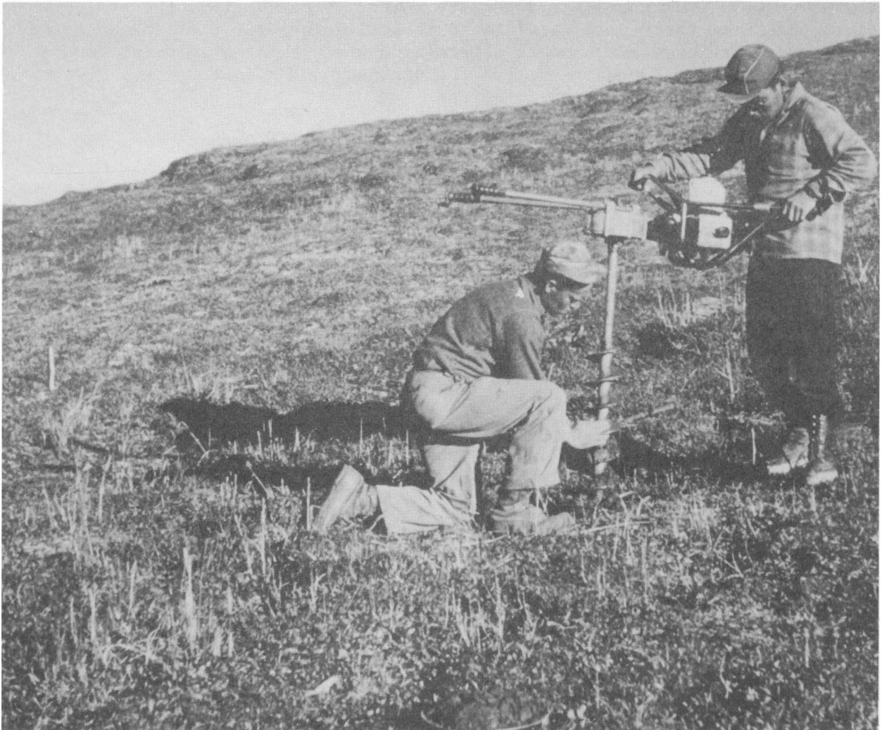
FIGURE 7. - Sampling Detrital Cover With a Gasoline-Powered Posthole Auger. The hole has been drilled, the auger is standing in a gold pan, and the kneeling man is scraping the sample from the scroll into the pan.
