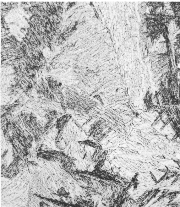
Figure 12. - Microstructure of press-forged material rolled at 850° C.-ingot 1. Kellers etchant.
