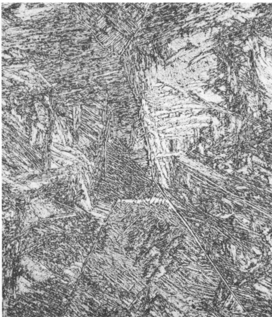
250 X Figure 18. - Microstructure of hammer-forged material rolled at 850° C.-ingot 2. Electropolish.
