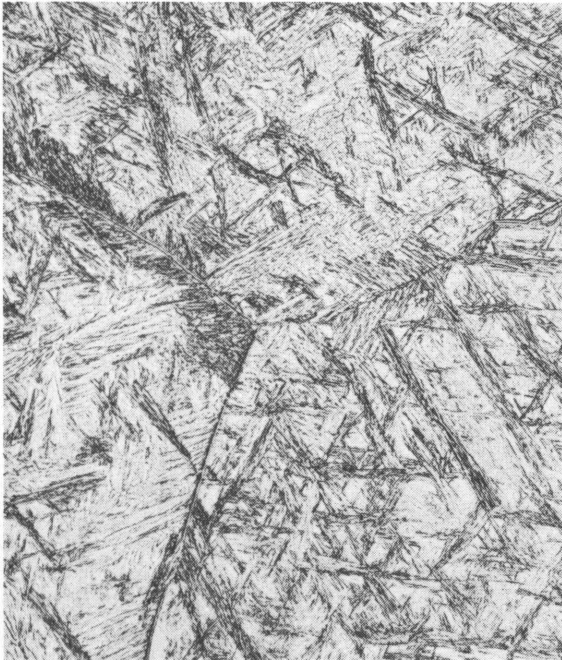
250 X Figure 16. - Microstructure of press-forged material rolled at 850° C.-ingot 2. Electropolish.
