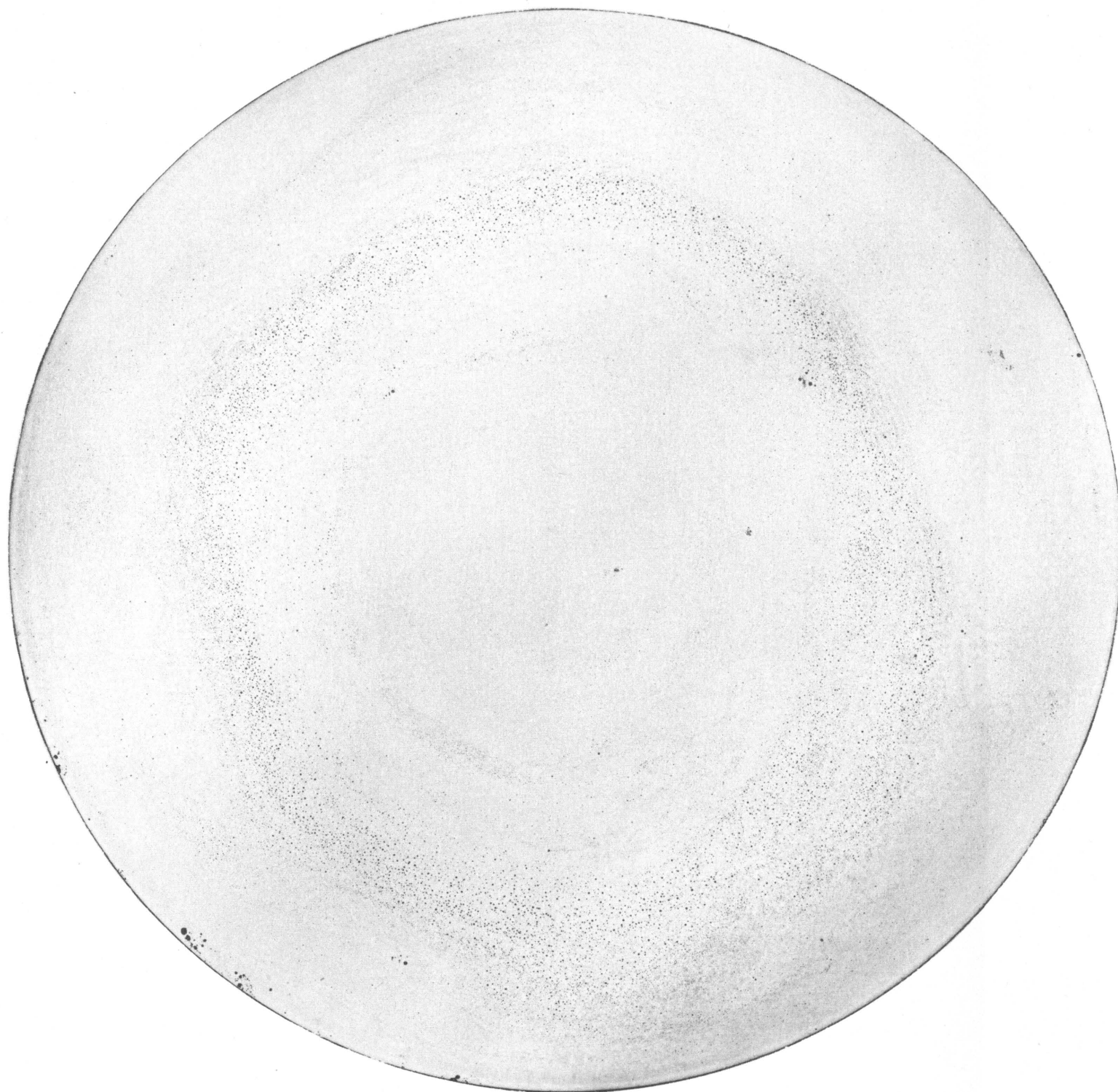
2/3 X Figure 3. - Polished cross section of heel of ingot 1.
