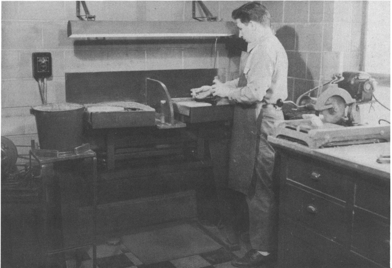
Figure 3. - This is a picture of the grinding machine and the operator beginning to condition the lap by grinding a quartz crystal. The container in the operator's left hand is the fine silicon carbide and water in a salt shaker. The bucket to the left of the grinding machine is the source for water used in grinding on the left grinding lap. The two cast-iron, 10-inch grinding laps revolve at 750 r.p.m. On the bench in back of the operator is the diamond saw used in cutting the rock slice.
