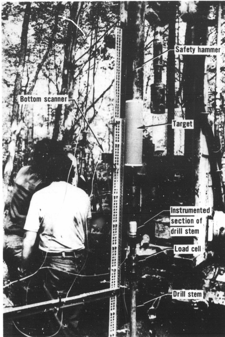
Figure 2-3. Photograph of test setup showing targeted safety hammer, instrumented section of drill stem, load cell, and top and bottom scanner opposite target. Angle frame is adjusted to be parallel to hammer prior to test.
