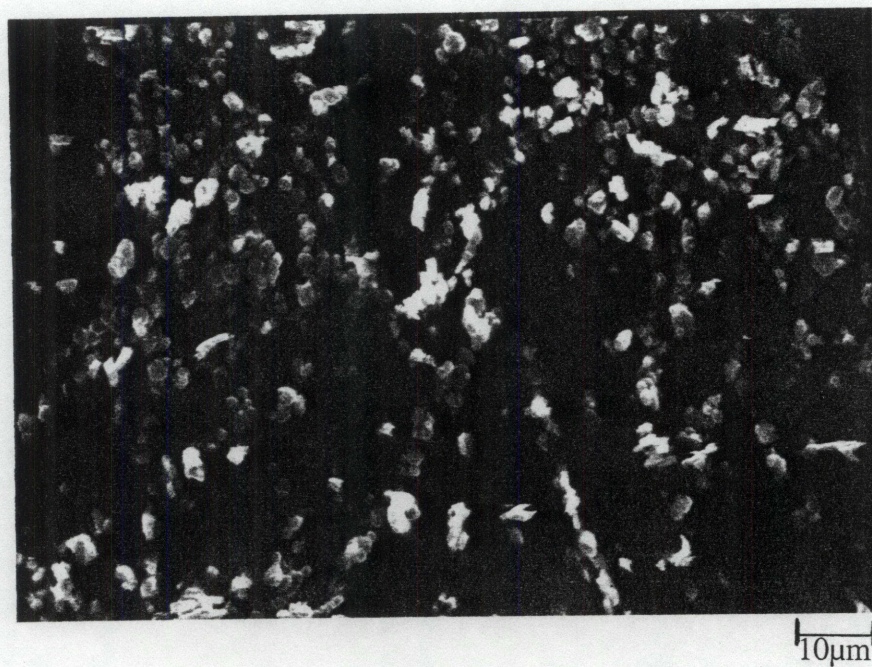
Fig 3.32 SEM of \text{Mg}_2\text{Al}(\text{OH})_6(\text{CO}_3)_{1/2} , from homogeneous precipitation by urea
