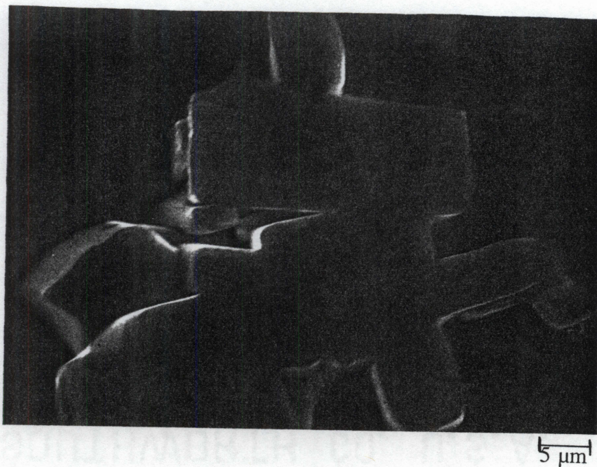
Fig 3.36 SEM of Mg 2 Al(OH) 6 Cl, annealed at 140°C in mother liquor for 1 week
