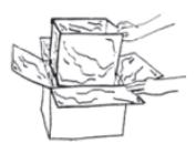
2. Add bottom supports and insulation. Cut out 4 cm squares from the discarded smaller box flaps. Glue them on top of each other to form eight pillars 2–3 cm high. Glue these pillars inside the bottom of the bigger box to support the inner box. Tear up newspaper sheets in fourths and crumple each piece into a lemon-sized ball. Cover the bottom of the bigger box with these balls.
