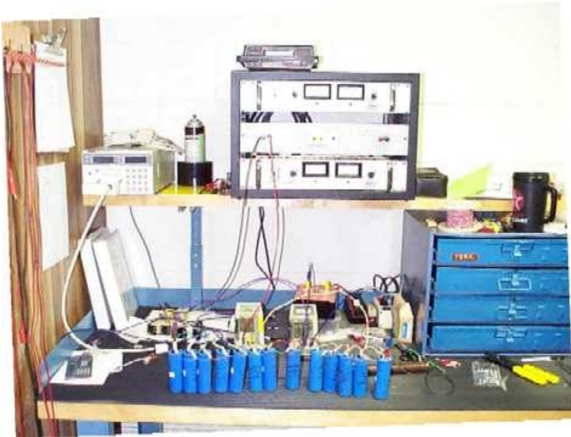
Figure 11, Reforming a group of 13 can style capacitors
