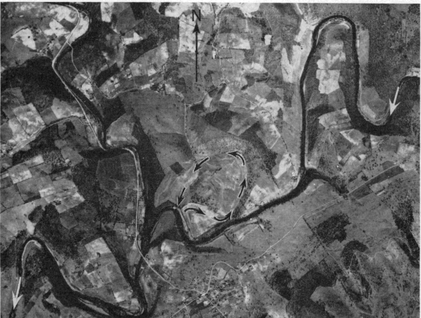
FIGURE 27. Aerial view of the cut-off meander at Woodway. Black arrows show the former direction of flow of the river around the abandoned meander.
