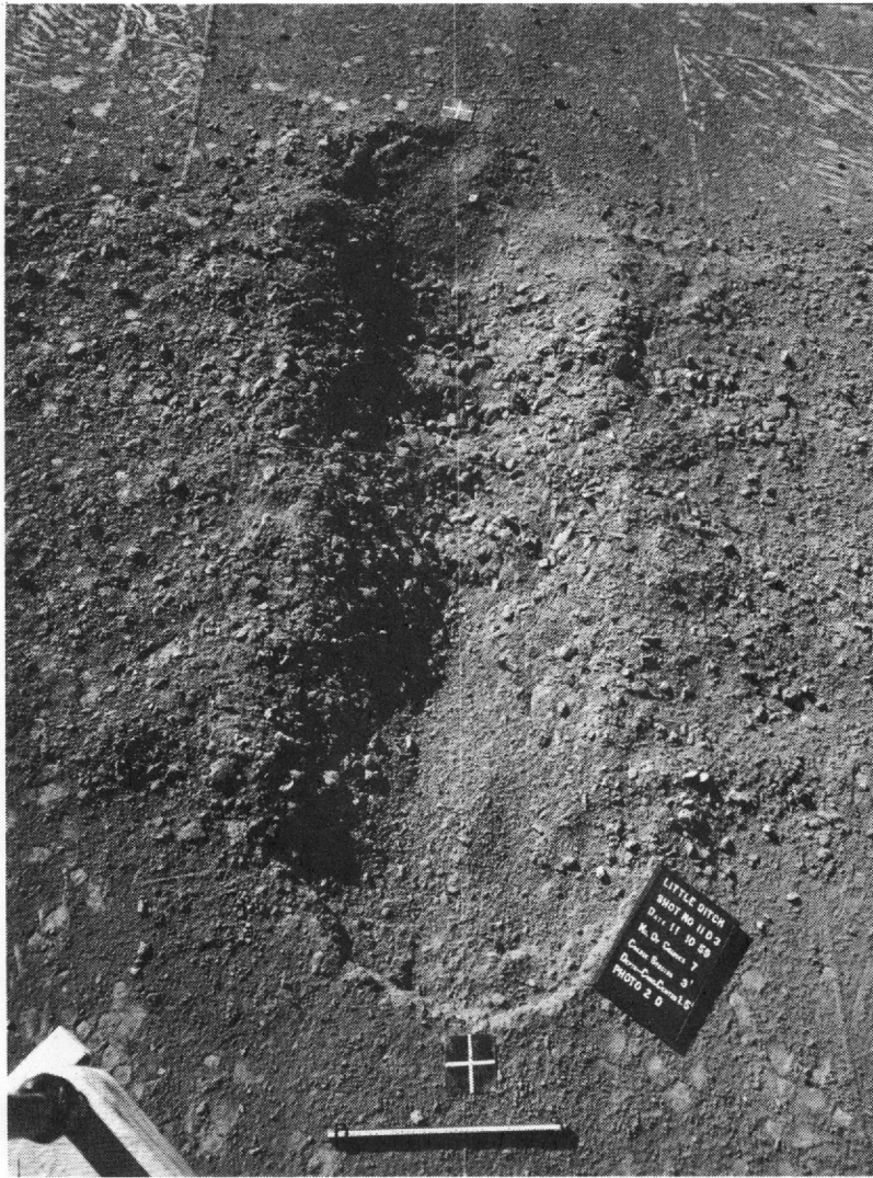
Figure 3.21 Typical row-charge crater showing absence of throwout off the end of the crater--seven 8-pound charges, buried 1.5 feet, spaced 3 feet apart
