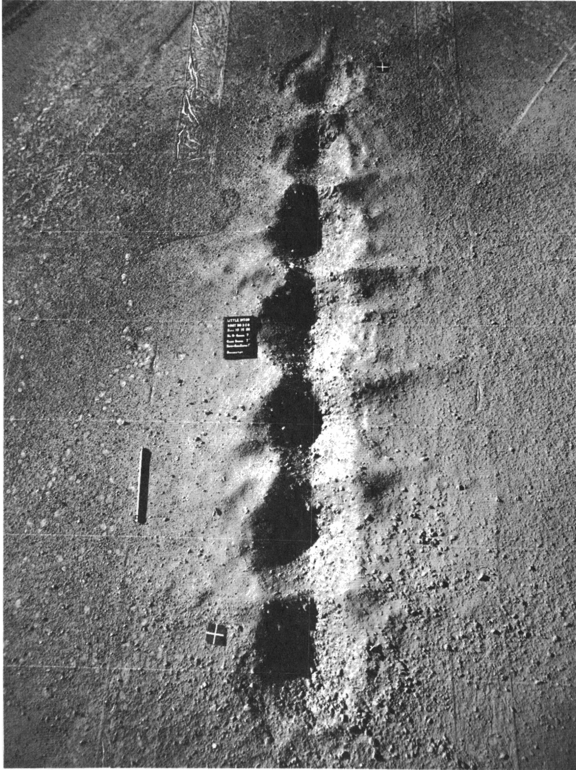
Figure 3.12 Typical row-charge crater in the region of line charge disparity--seven 8-pound charges buried 1 foot, spaced 7 feet apart
