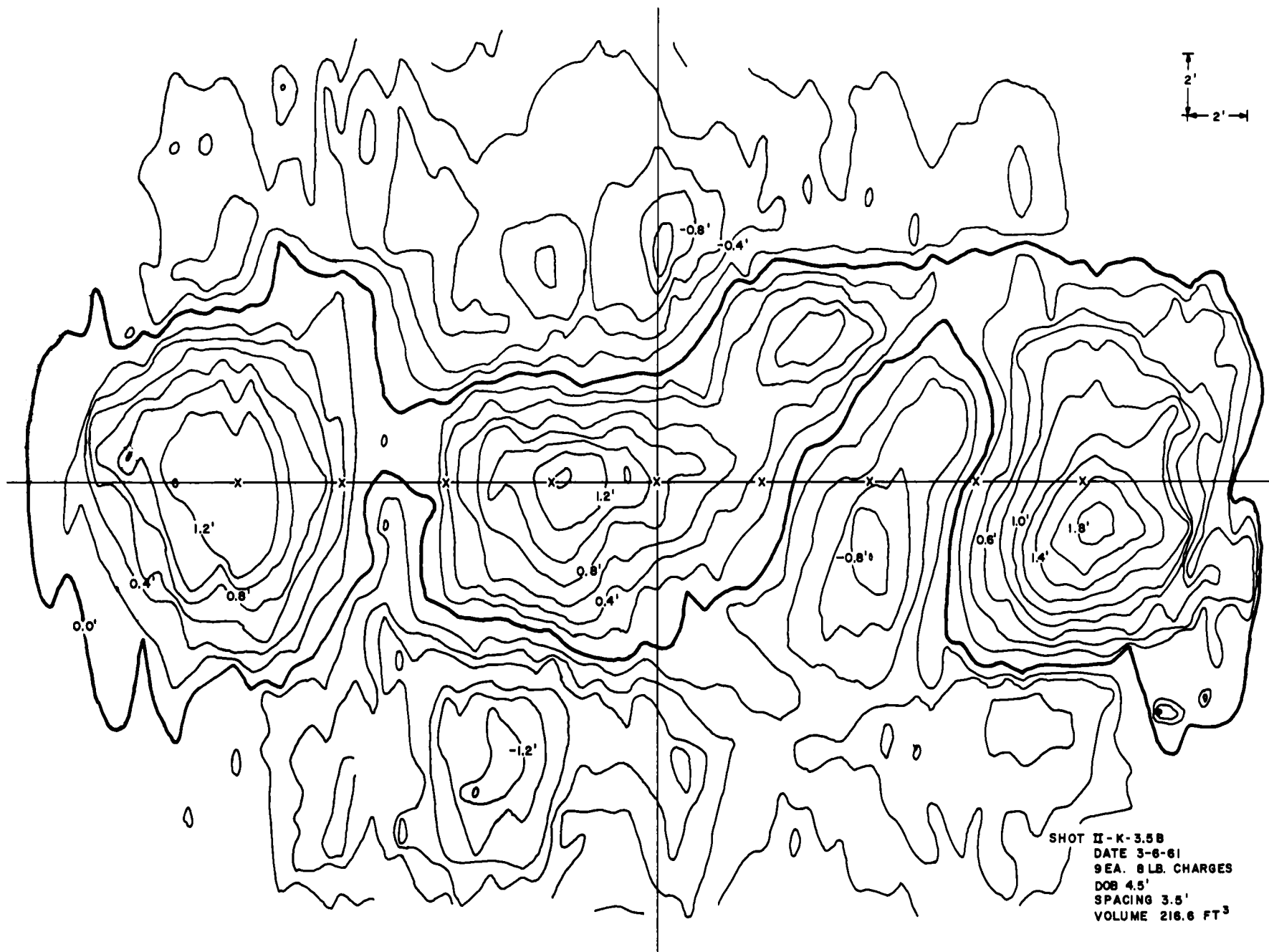
Figure B.33 Crater topography 8-pound row charge buried 4.5 feet, spaced 3.5 feet
