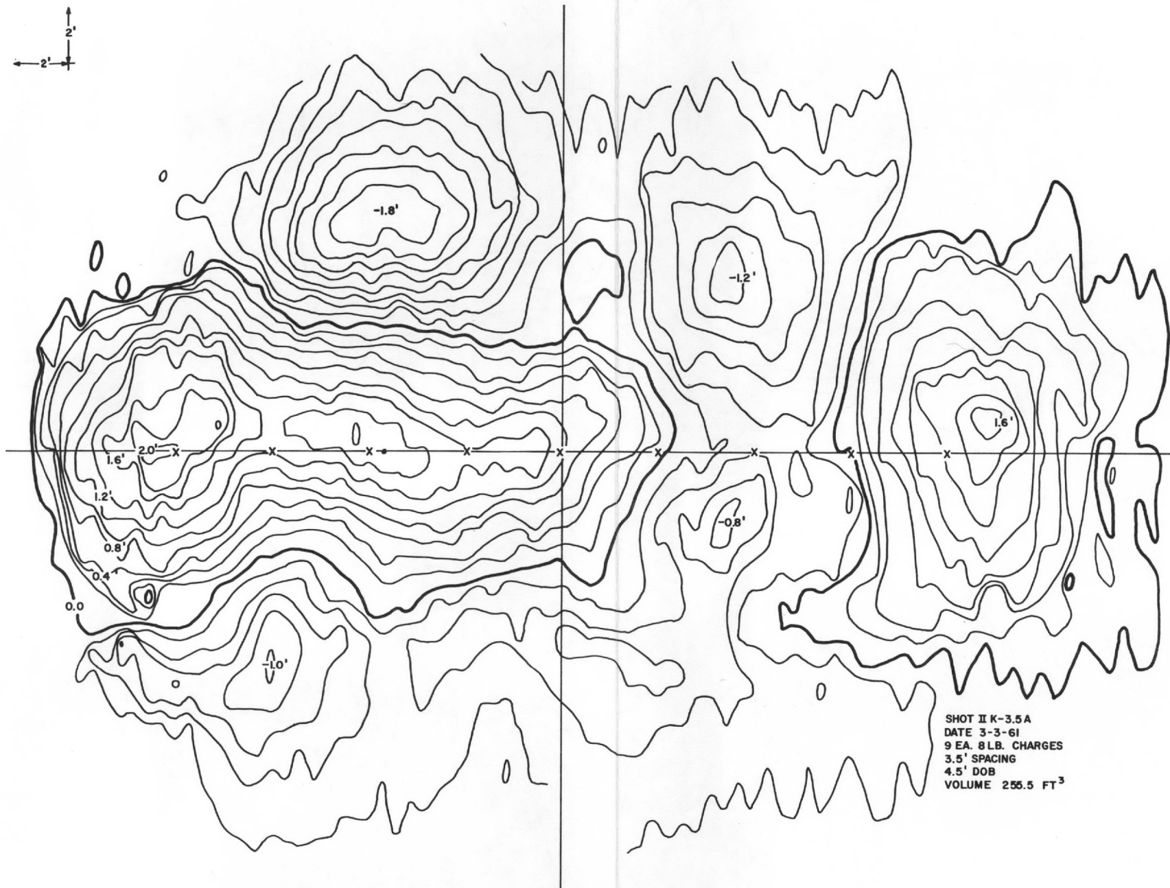
Figure B.32 Crater topography 8-pound row charge buried 4.5 feet, spaced 3.5 feet
