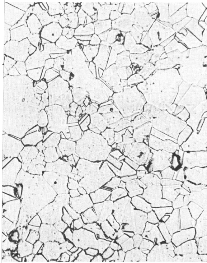
Fig. 3.1-4 – Optical micrograph of unshielded A-286
