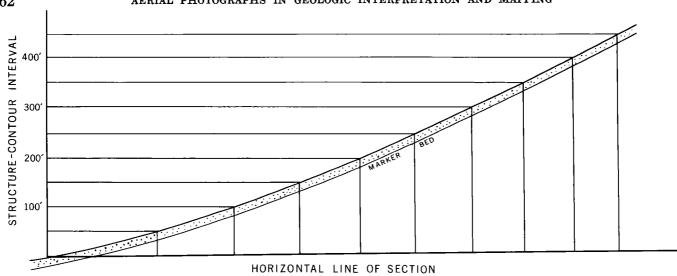
Figure 30.—Diagram showing graphic construction in positioning structure-contour lines on top of marker bed and the projecting of these lines to their relative horizontal positions along the line of section.
