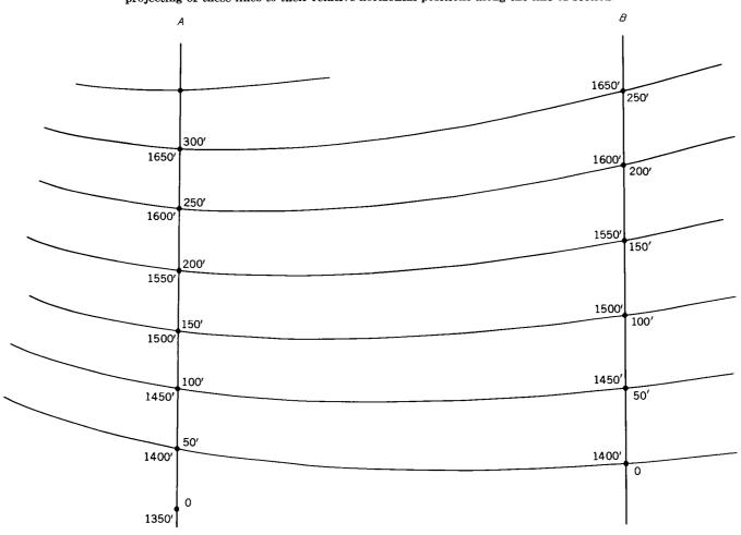
FIGURE 31.—Diagram showing relation of structure-contour positions along two lines of section at different altitudes.
