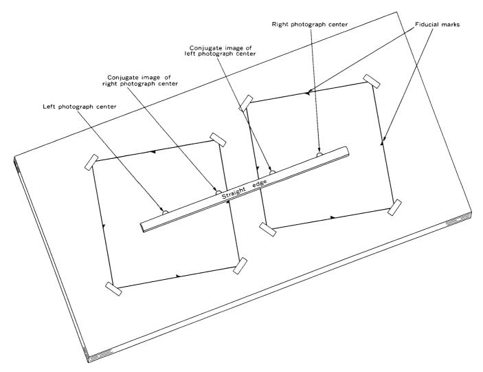
FIGURE 25.—Sketch showing correct orientation of photographs for stereoscopic viewing.
