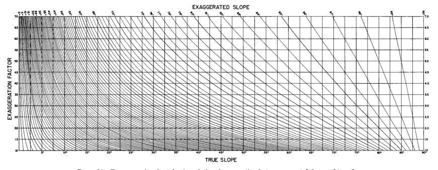
FIGURE 34.—Slope-conversion chart showing relation of exaggeration factor, exaggerated slope, and true slope.
