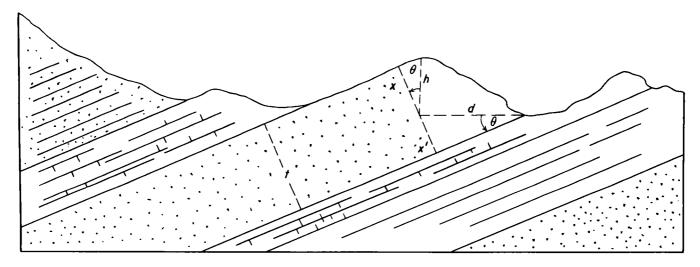
FIGURE 26.—Diagram of gently dipping beds showing relation of stratigraphic thickness to differential parallex determined at any two points along dip direction and at the formation contacts.
