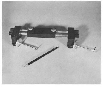
FIGURE 33.—Stereo slope comparator.
