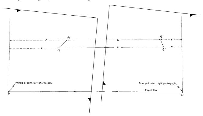
FIGURE 23.—Diagram showing relation between absolute stereoscopic parallaxes and horizontal distances actually measured with stereometer-type instruments in determining differences in altitude from paper prints.
