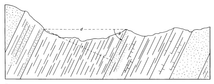
FIGURE 28.—Diagram of steeply dipping beds showing relation of stratigraphic thickness to dip angle and horizontal distance between top and botton of bed.
