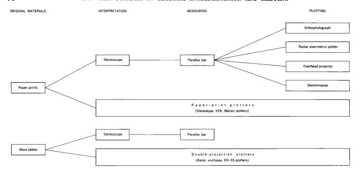
FIGURE 36.—Photogrammetric systems for geologists.
