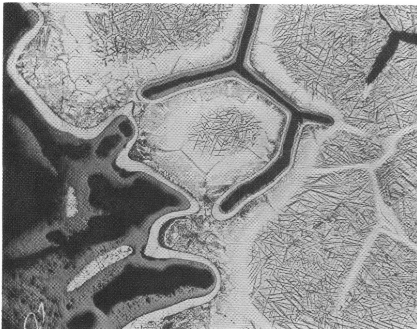
Figure 162. Structures near the surface of an exposed vanadium-modified ZrH-uranium fuel sample
