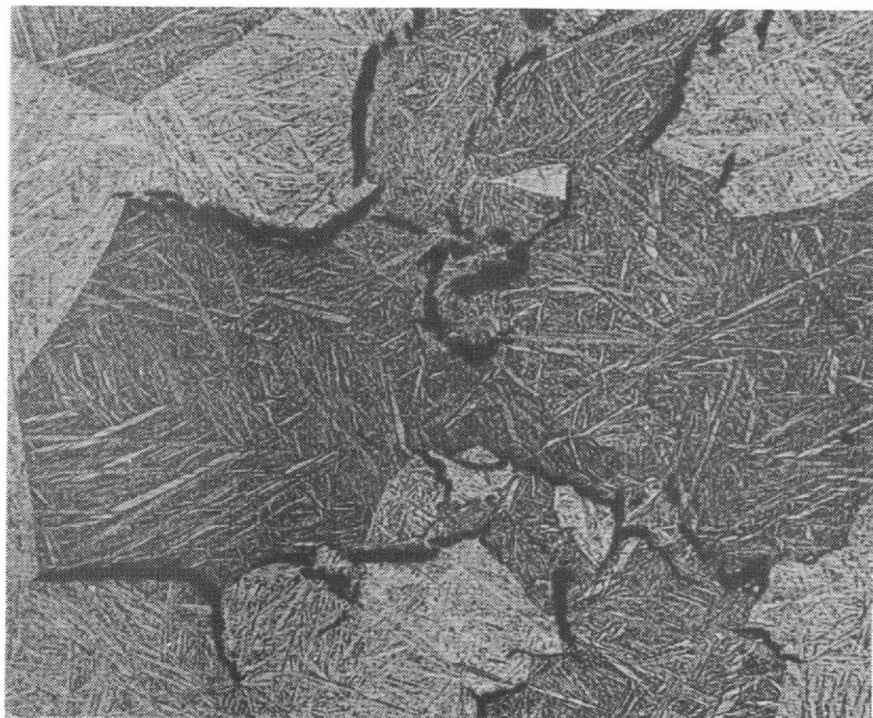
Figure 158. Voids in the interior of an exposed tin-modified ZrH-uranium fuel sample
