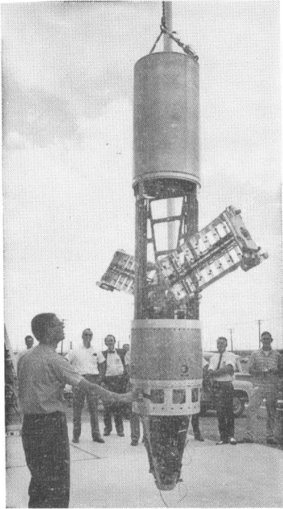
Figure 94. SAND-LO rocket sampler being developed by Sandia Corporation--beginning of blade extension
