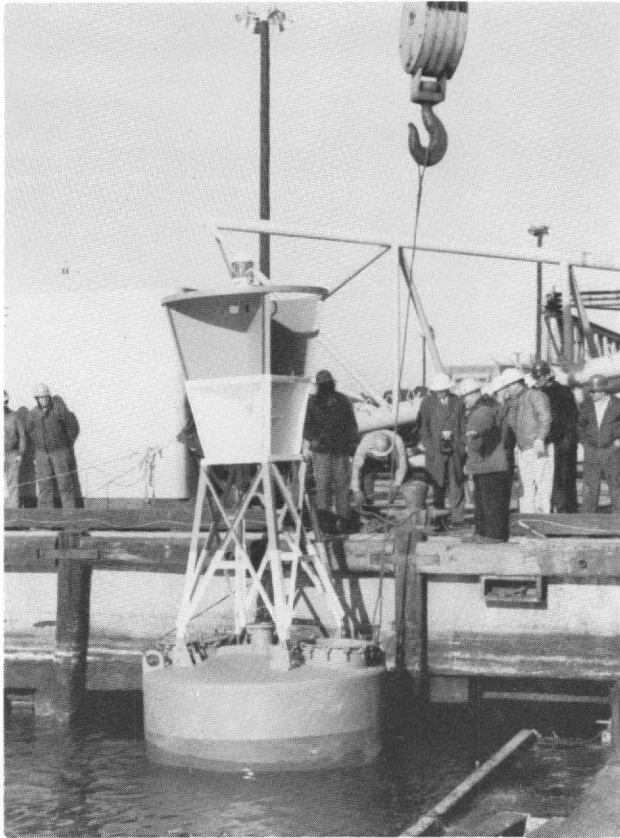
Fig. B-20, Light Buoy with SNAP 7A Generator Is Launched at Coast Guard Pier
