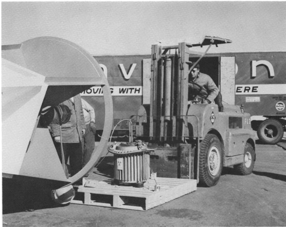
Fig. B-11. SNAP 7A Generator Is Transported from Moving Van to Coast Guard Buoy
