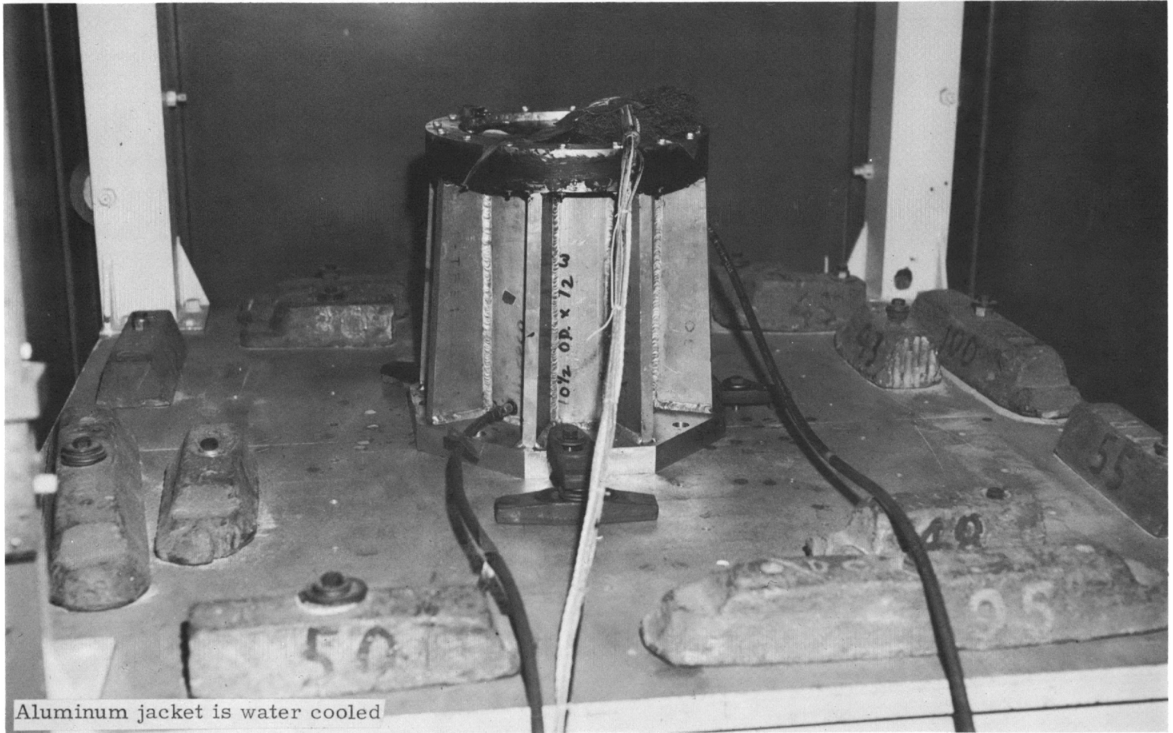
Fig. 43. SNAP 7A-7C Thermoelectric Generator Positioned on Barry Medium Impact Shock Machine for Vertical Shock Tests
