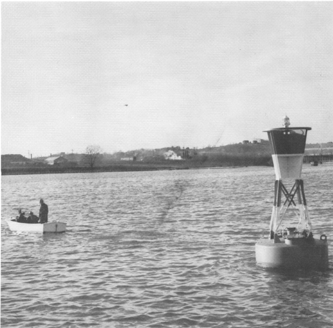
Fig. B-22. Light Buoy with SNAP 7A Installed Is Towed to Mooring Test Site
