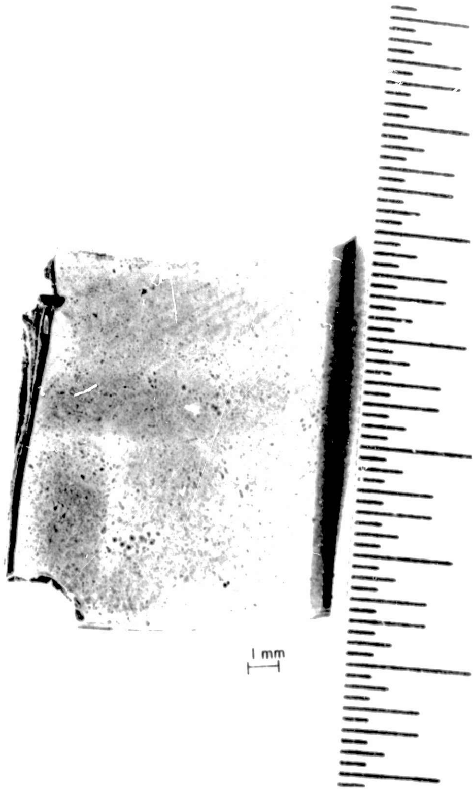
Fig. 51. Enlarged View of Fracture Surface and Gouged Area of HYGAS Valve Assembly Leaf Spring. ANL Neg. No. 306-77-547
