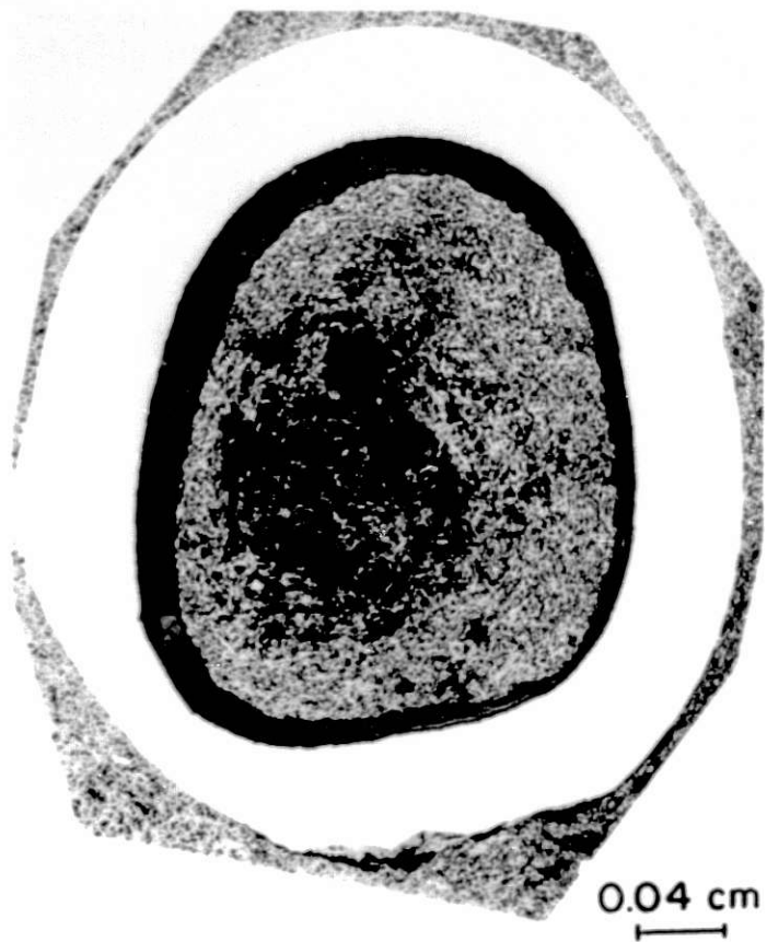
Fig. 77. Optical Photograph of a Cross Section of the Taphole Cooling Coil. A corrosion scale is seen at the ID, and localized corrosion is visible at the OD. Neg. No. ANL-306-78-575
