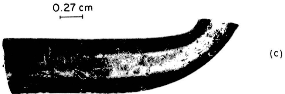
Fig. 76. Optical Photographs of the Taphole Cooling Coil: Overall view (a), Cross-sectional View (b), and Top View (c). The tube ID is out of round, and the outer surface contains many imperfections. ANL Neg. No. 306-78-572
