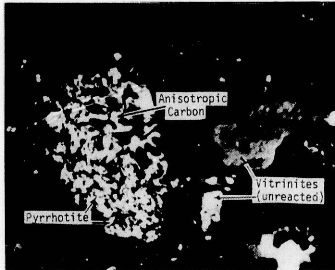
Hot-Separator Coke (P99-66)
