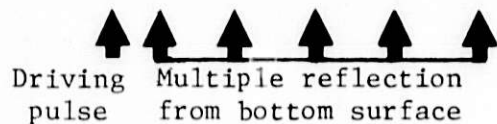
Fig. 17. Multiple Ultrasonic Reflections from Bottom Surface of Al Test Block as Received by EMAT.
