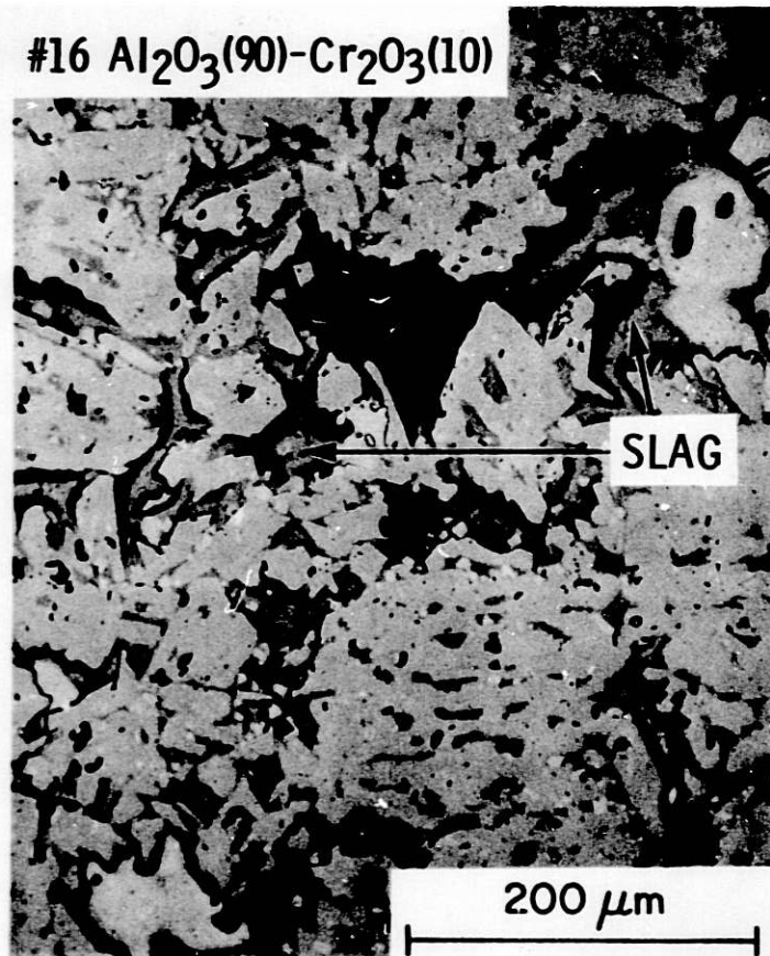
Fig. 5. Reflected-light Image \sim 1 mm from the Slag-Refractory Interface of Number 16, Showing Intergranular Attack.
