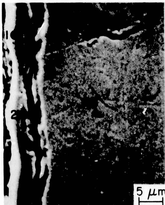
Fig. 24. SEM Photomicrograph of Incoloy 800 Specimen Preoxidized at p_{O_2} = 9.2 \times 10^{-18} atm and Subsequently Sulfidized at p_{S_2} = 2.9 \times 10^{-13} atm. The elemental analyses for regions 1 through 3 are given in Table II.
