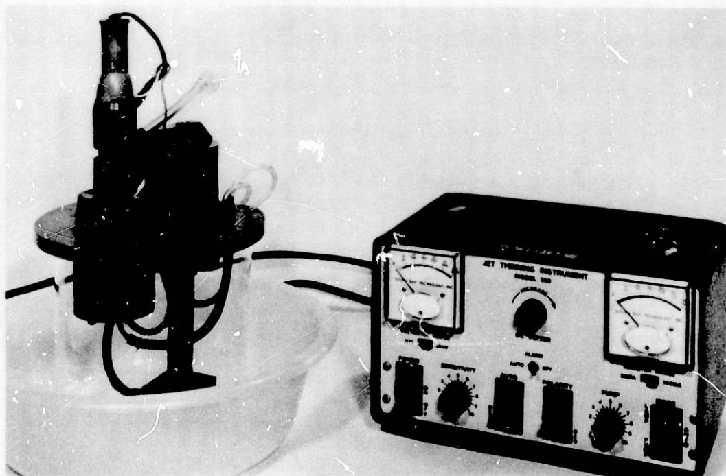
Fig. 3. Apparatus for Jet Electropolishing. ANL Neg. No. 306-80-234.
