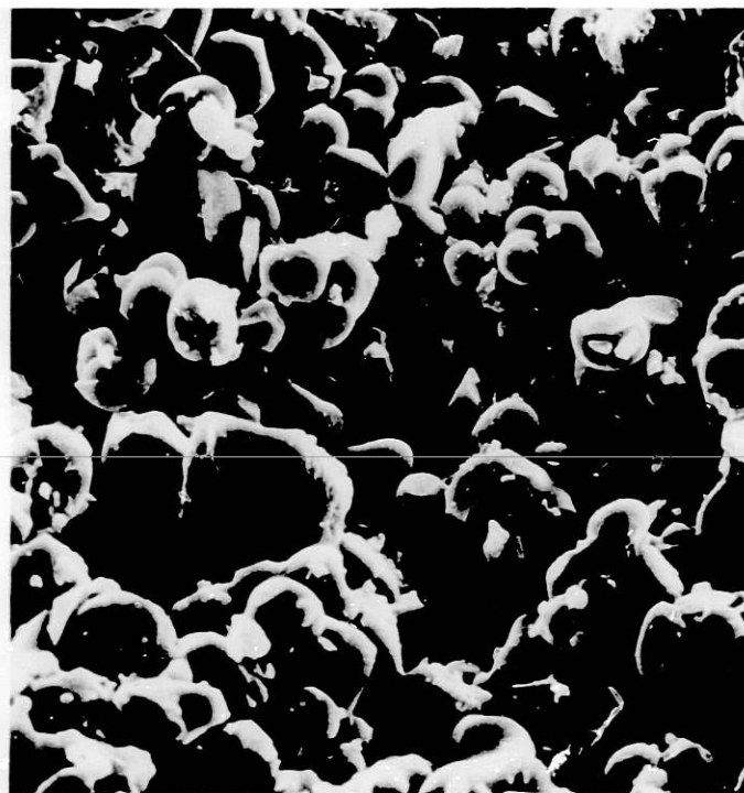
Fig. 4. Microstructure Typical of Sintered \text{LiAlO}_2 Prepared from Batches 134-82 and -83 Containing Uniformly Large Particles. (Magnification, 1500X.)
