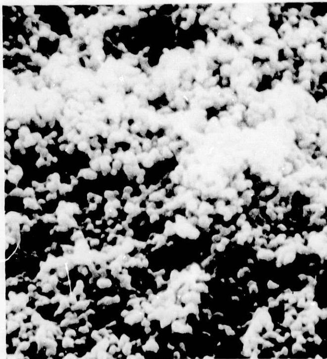
Fig. 1. Microstructure of Sintered \gamma -LiAlO 2 from Batch 134-63 Containing Uniformly Small Particles. (Magnification, 12,000X.)
