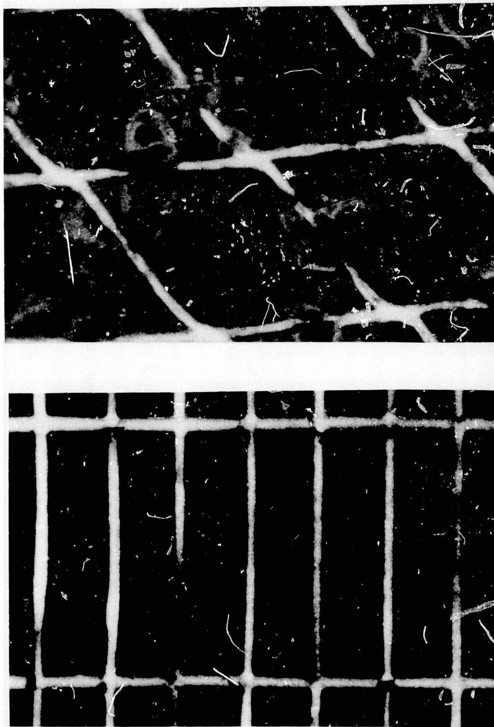
Fig. III-3. Radiographs of a Pb-Ca Expanded-Metal Grid (top) and a Pb-Sb Cast Grid (bottom) Showing Different Locations of Corrosion
