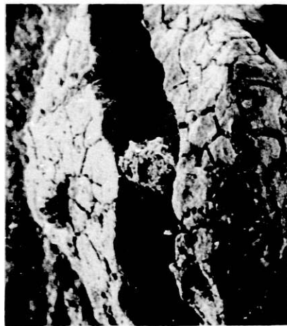
WHOLE ROCK PHOTO HYDRATED, PARTIALLY-SULFATED COMBUSTOR LIMESTONE FEED MATERIAL 132X
