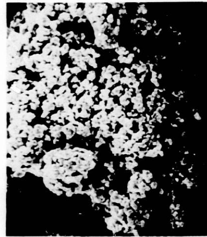
CLOSE-UP OF \text{Ca(OH)}_2 CRYSTALLITES 3300X
