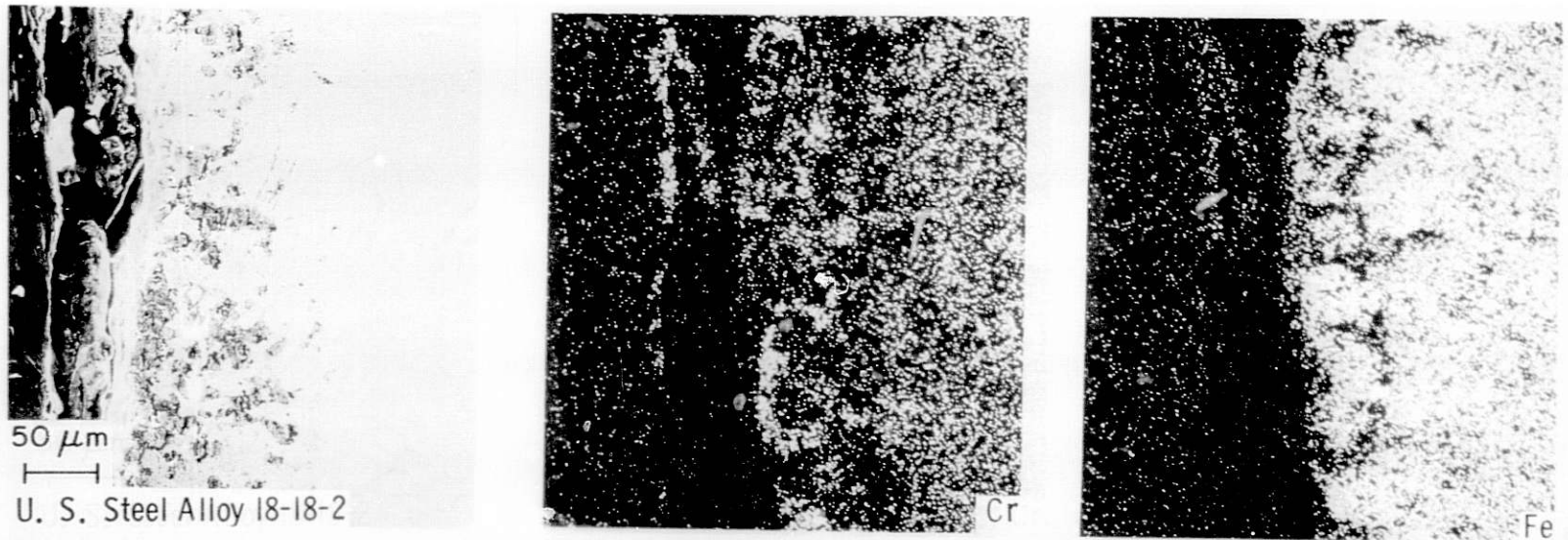
Fig. 34. X-ray Photograph and Cr, Fe, Ni, Si, and S Distribution in U.S. Steel Alloy 18-18-2 Specimen After a 3.6-Ms Exposure to a Complex Gas Mixture at 871°C (Run D03B871). In the distribution pictures, light regions indicate a high concentration of the respective elements. ANI, Neg. No. 306-79-325.
