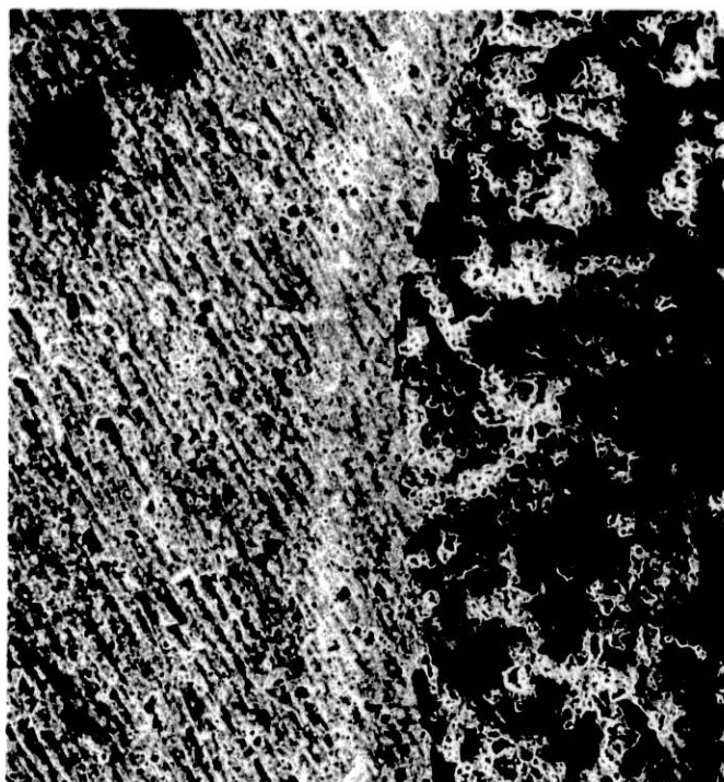
Fig. 17. Photographs of Agglomerated Simulated (PW-7a) Spray Calcine Mixed with 15 wt % Glass Frit Granules (sintered at 1050°C) and Dispersed in a Lead Matrix: (a) 12X with optical microscopy (b) 24X on SEM, and (c) 110X on SEM
