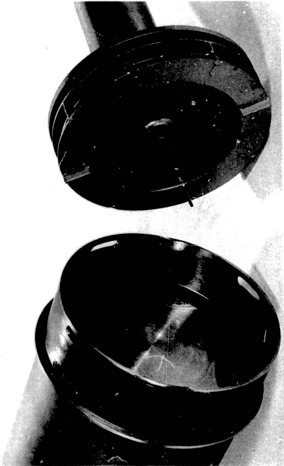
Fig. 8. Upper Zone of 0.5 Mg/d Centrifugal Contactor Showing Weirs. ANL Neg. No. 308-77-593
