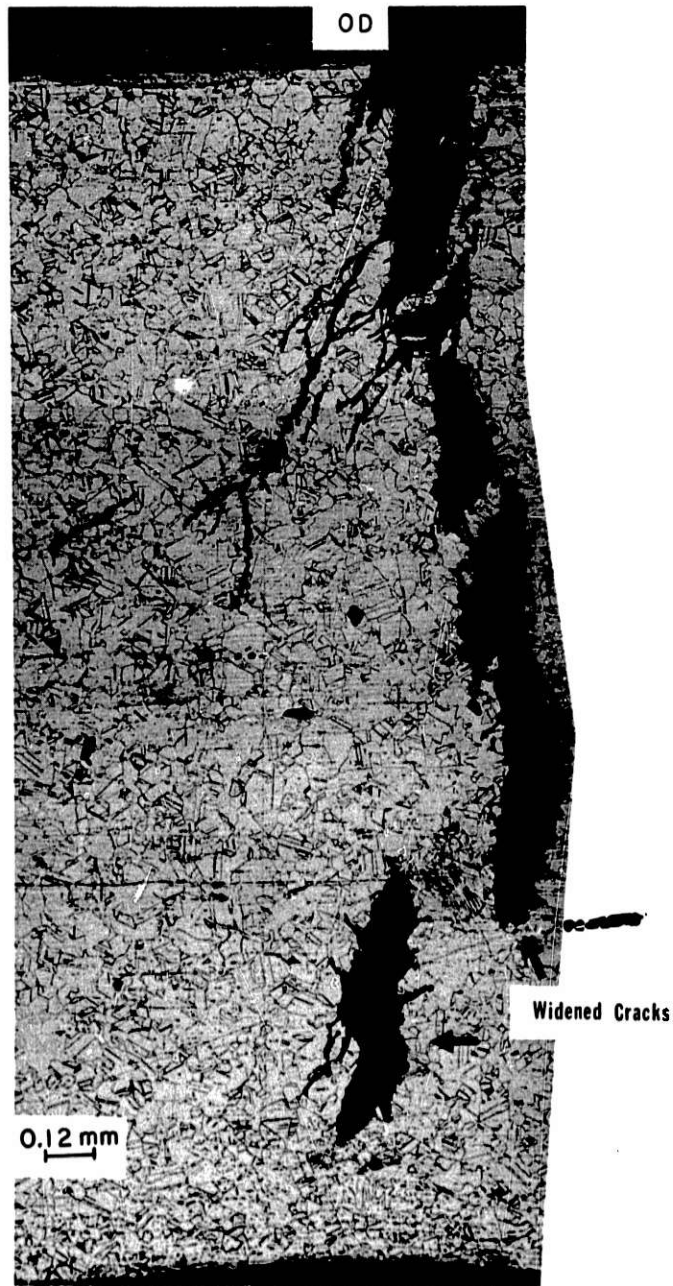
Fig. 48. Cross Section of 6411. Transgranular and branched cracks are visible. ANL Neg. No. 306-78-41.
