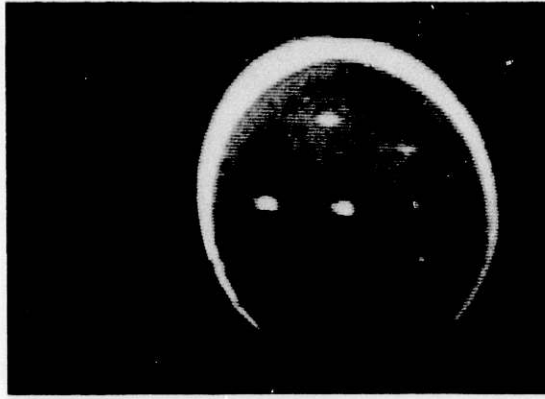
Fig. 22. Transaxial Spin-Echo NMR Image of an MgO/20% Polyethylene Glycol Green Ceramic Compact with the Hole Pattern Shown in Fig. 21. Benzene was used as the filler fluid. The bright rim is pure benzene. The bulk of the ceramic body exhibits an NMR-derived porosity of 15.5 \pm 6.2\% , and the dark, round patch has a porosity of 7.4 \pm 1.7\% . The background (noise) value is 2.1 \pm 1.1\% .
