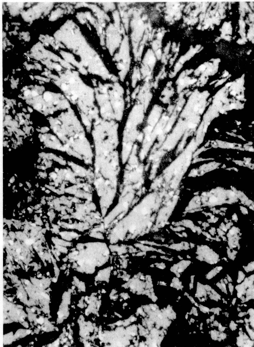
Fig. 19. Photomicrograph of \text{Li}_2\text{FeS}_2 (light gray) and \text{Fe}_{1-x}\text{S} (white). (650X)
