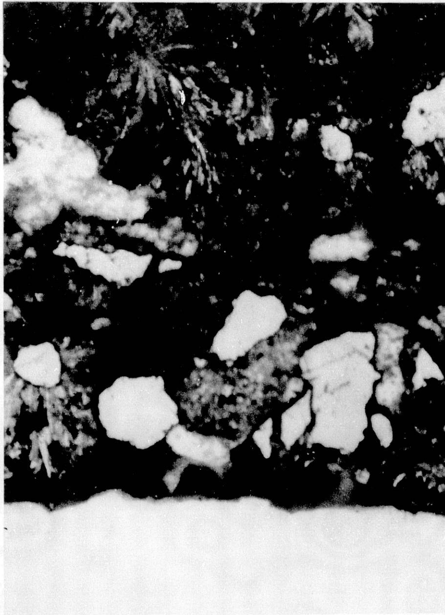
Fig. 22. Photomicrograph of \text{FeS}_2 Particles (light) and Discharge Products (dark) Randomly Distributed through Positive Electrode of Cell PC036. (Areas containing the electrolyte-MgO mixture appear hazy white.) (130X)
