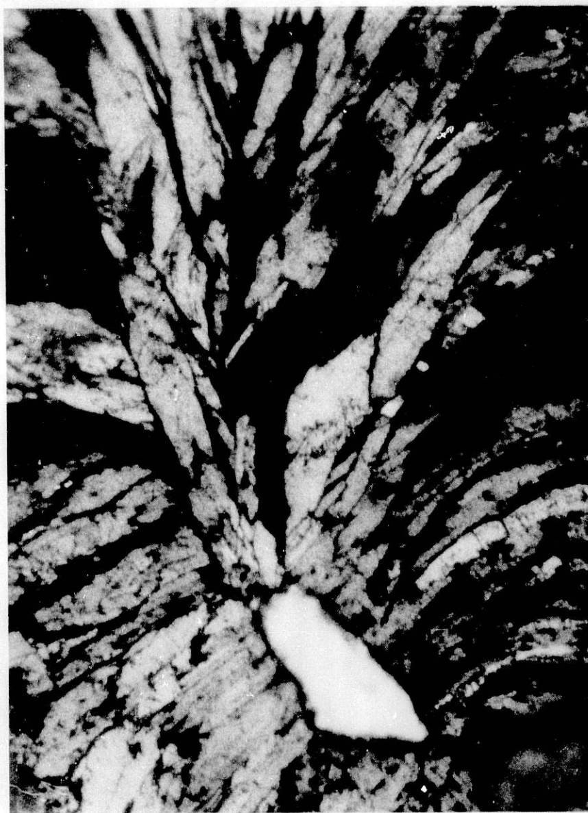
Fig. 18. Photomicrograph of \text{FeS}_2 (white) and \text{Li}_3\text{Fe}_2\text{S}_4 (light gray). (650X)
