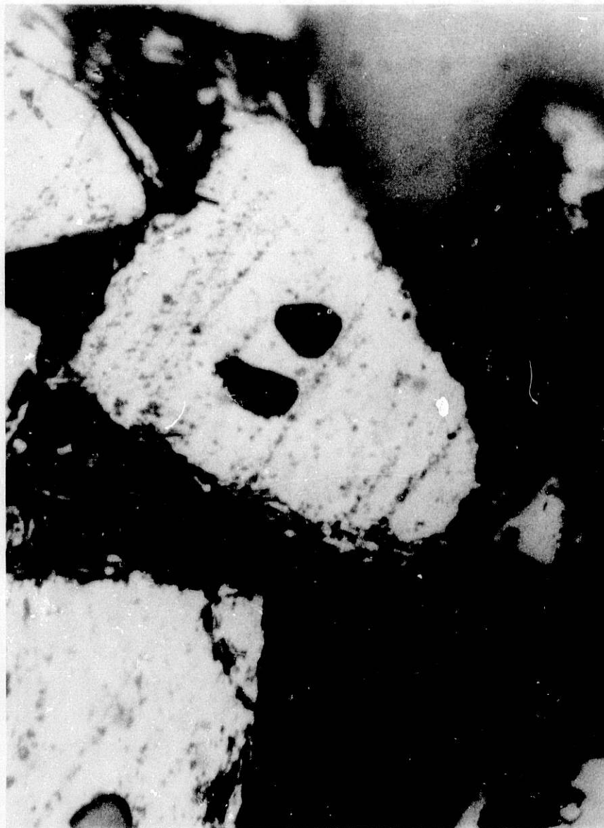
Fig. 17. Photomicrograph of Coarse \text{FeS}_2 Particle Containing \text{SiO}_2 . (650X)
