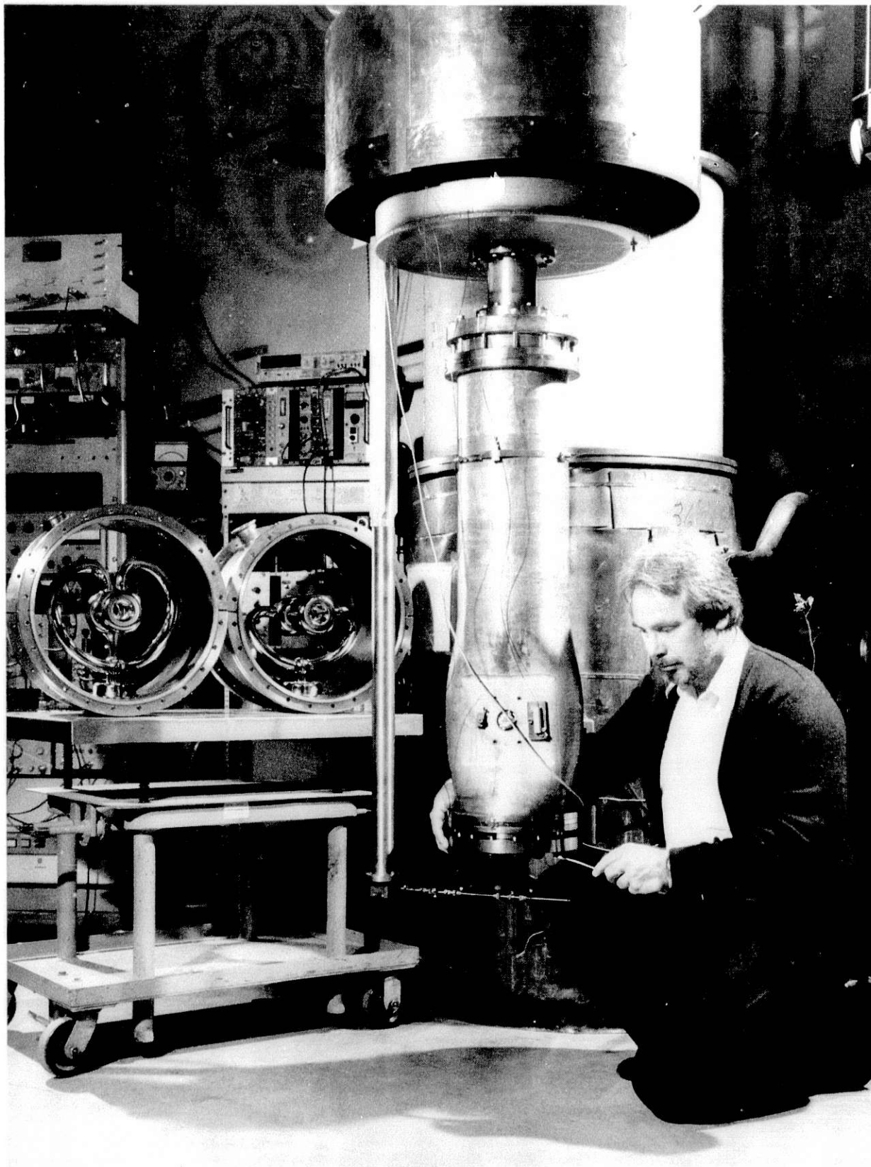
Figure IV-2. Ken Shepard with the first prototype of his superconducting interdigital accelerating structures. The split-ring resonators used in ATLAS are on the left.
