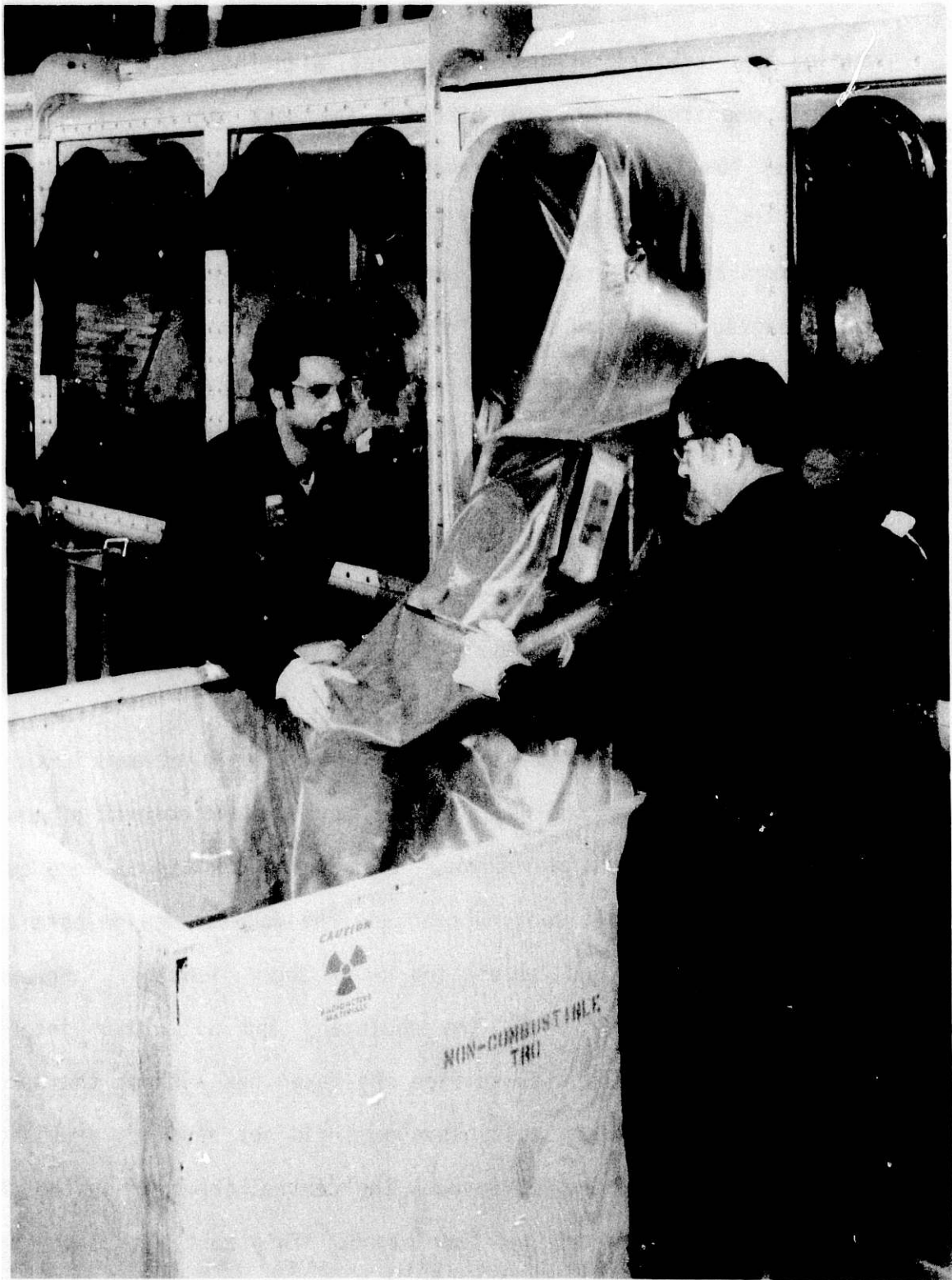
Figure 4-11 Bagging Waste Out of a Glovebox
