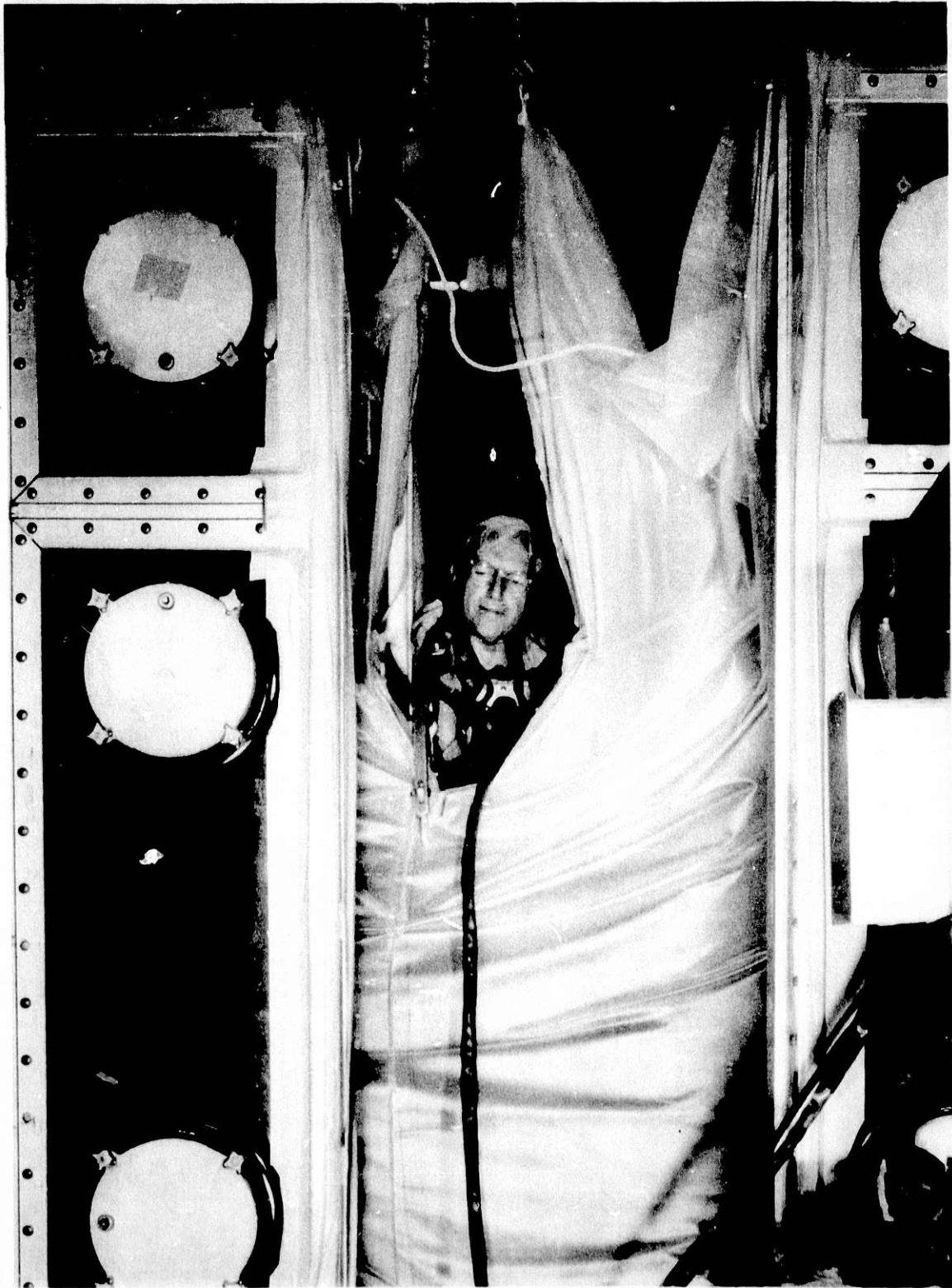
Figure 4-6 Heat Sealing Glovebox Separation Pouch
