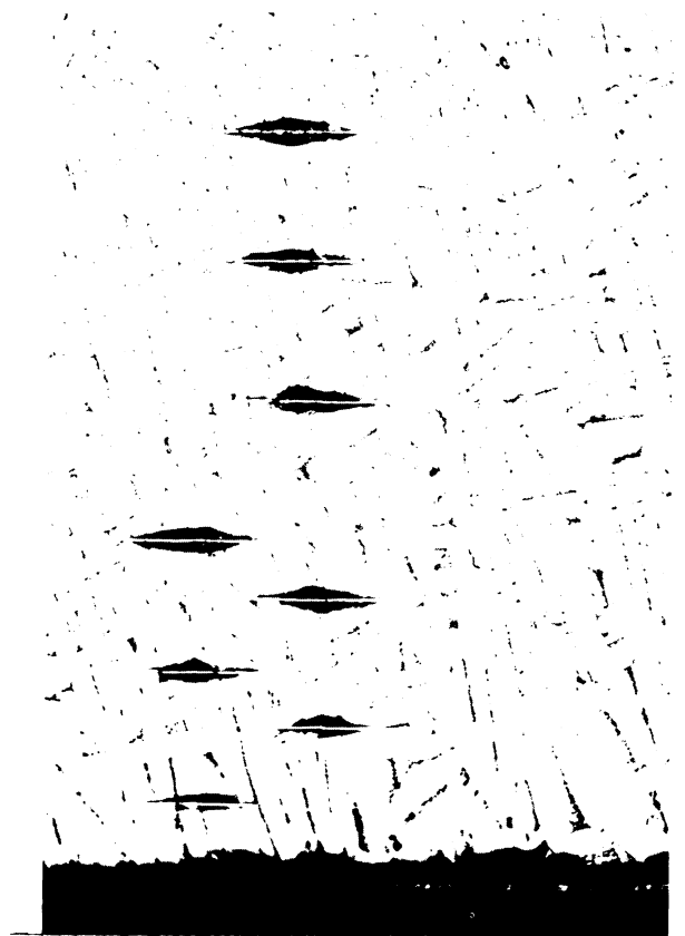
Figure 142.—Microstructure of zirconium cast in mold material BW near cast surface (SA 21,674). Etch: 45 ml H 2 O, 45 ml HNO 3 , 10 ml HF ( \times 100 ).
