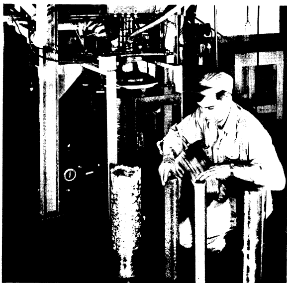
Figure 3.—Melting section of furnace with consumable pressed electrodes and ingots in foreground.
