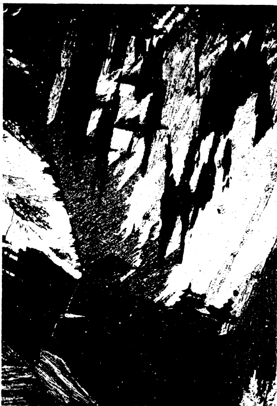
Figure 137.—Microstructure of titanium cast in XM-76 near cast surface. Etch: 45 ml H 2 O, 45 ml HNO 3 , 10 ml HF ( \times 50 ).
