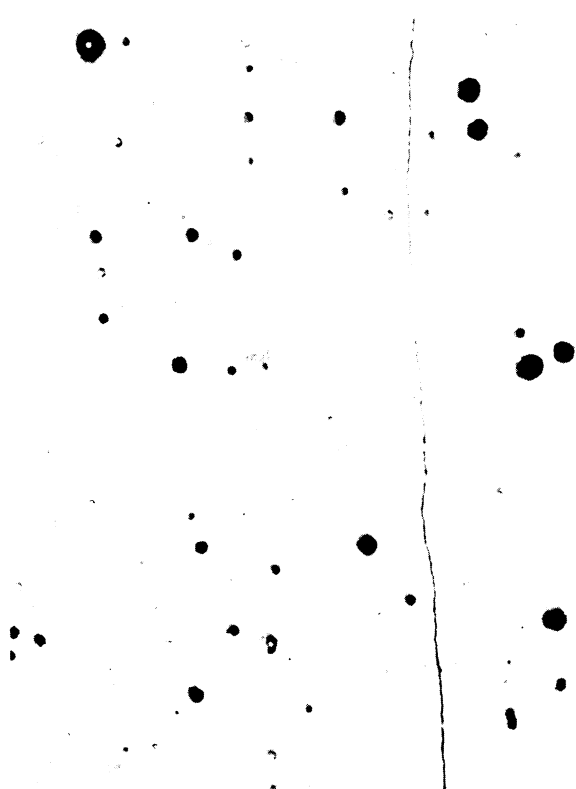
Figure 25.—Photomicrograph of electrolytic cathode copper vacuum-arc-melted in water-cooled copper crucible ( \times 250 ).
