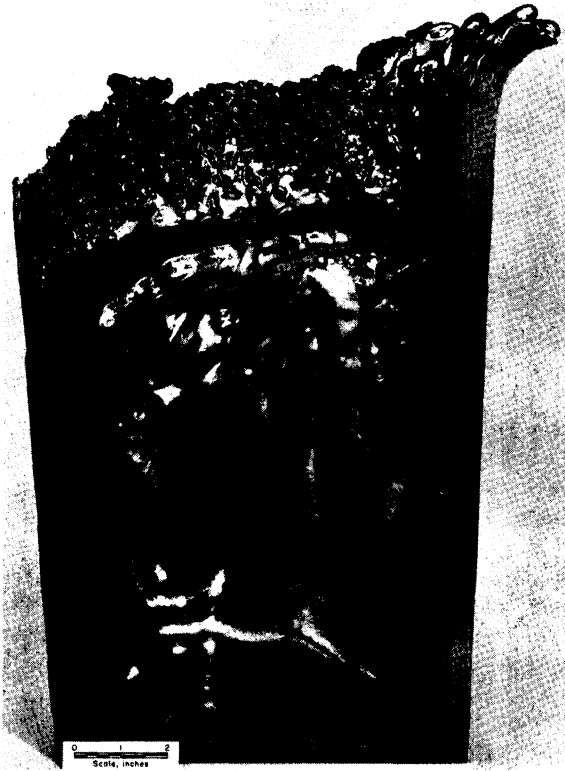
Figure 48.—Skull of zirconium remaining in the crucible of a consumable electrode arc melting and casting furnace after pouring.
