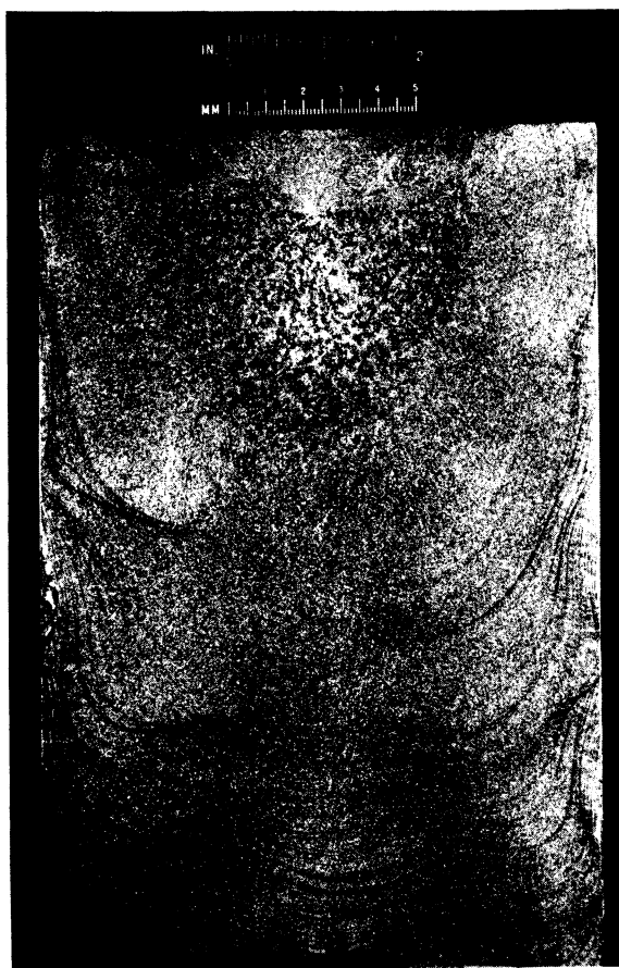
Figure 6.—Single melt ingot using 1.4 amp for solenoid stirring causing centrifuging of tin to sidewalls.
