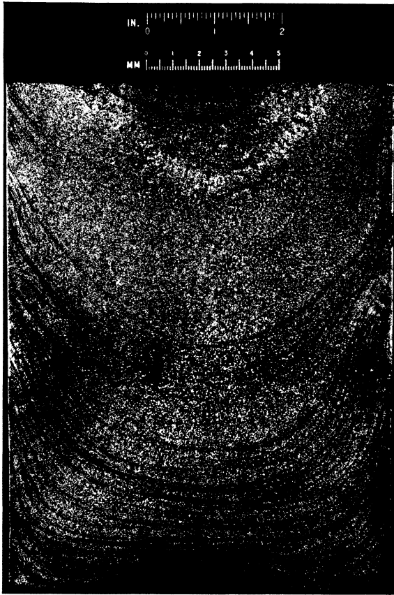
Figure 7.—Single melt solenoid stirred ingot of 0.2-amp type.
