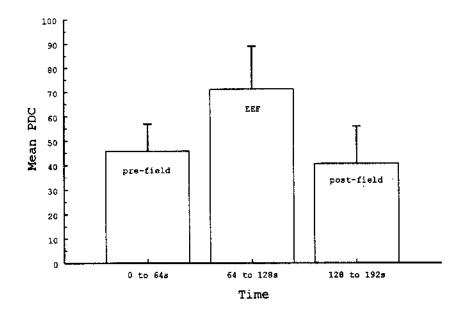
Fig. 9. Effects of an EEF (d.c.: 90V/cm) on the mean variation in light transmittance (PDC) in 10 isolated crayfish nerves pretreated with TTX (10mM) for 1 minute.
