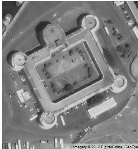
Figure 9. Forte Michelangelo, Civitavecchia, Italy. The polygonal bastion on the northern end of the fort bearing the name of one of its architects, Michelangelo, exemplifies the trend toward what would become the trace italienne . However, the round towers show a lack of full deployment of an angled bastion and still result in dead zones. Source : Google Maps.
