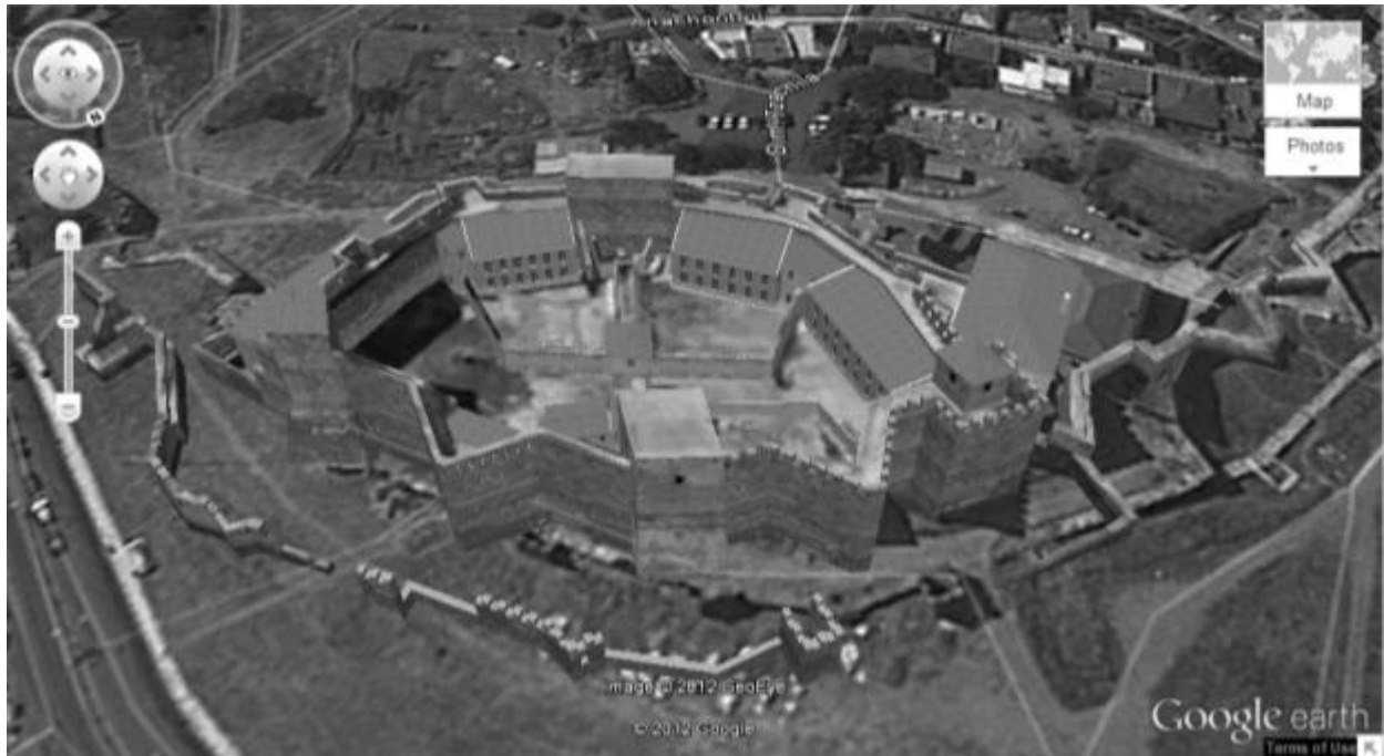
Figure 27. Heptapyrgion at Thessaloniki. Note the triangular towers that provide a flanking defense of the wall and potentially the square towers while allowing. Also note that the triangular towers are covered from multiple angles from adjacent towers and the curtain. Additionally, the triangular towers on the outer wall over on the right hand side of the image show the continuation of the same pattern on the rest of the walls. It is probable that the triangular towers of the Heptapyrgion are based on the pattern seen in the triangular bastions of the outer city wall. Source: Google Earth.
