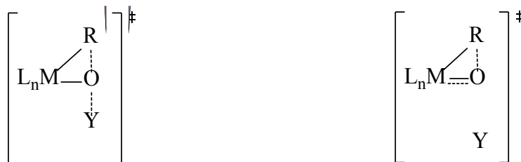
Figure 5.11. Proposed connection between Baeyer-Villiger and oxo pathways for oxy-insertion ( MR + [O] \rightarrow MOR ) where M = metal, R = alkyl or aryl transfer group, Y = leaving group, and L_n = ancillary ligand.
