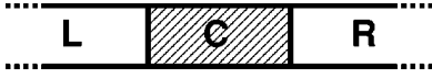
FIG. 1. A conductor described by the Hamiltonian H_C , connected to leads L and R , through the coupling matrices h_{LC} and h_{CR} .
