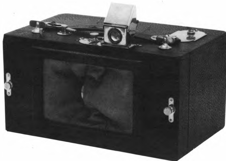
Figure 9. Model 4G Al-Vista of 1903. Notice the top lever film punch instead of side bottom film punch on previous Al-Vistas.
