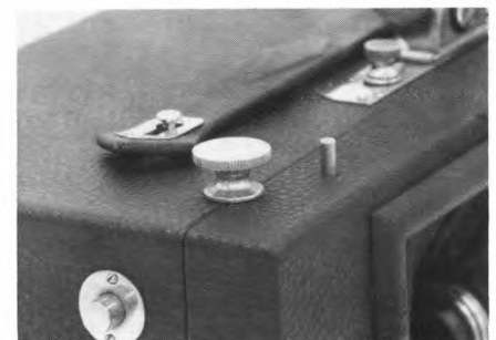
Figure 4. Knurled type winding knob on 1900-1901 Al-Vistas.
