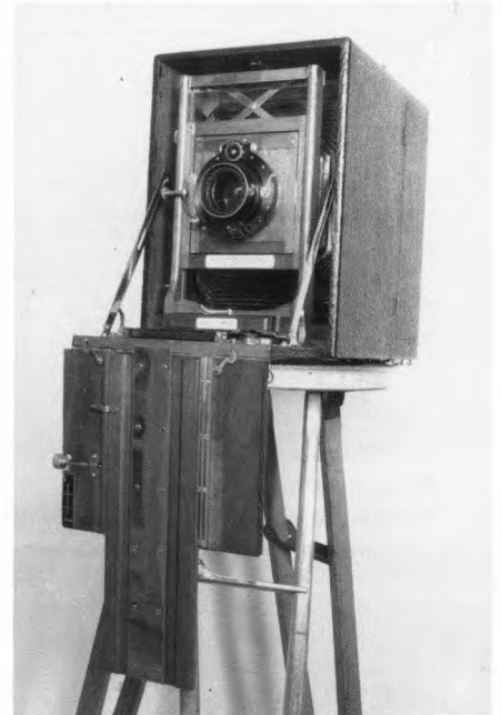
Figure 5. A modified Model I showing the front bed drop provision where a 6" auxiliary bed is installed for the camera lens frame to slide on for focusing.
