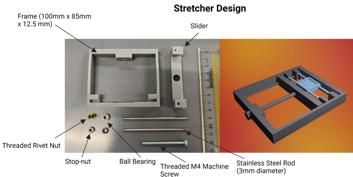
Figure 2.1: Overview of components that comprise the stretcher platform (left) and a computer model of the assembled platform (right). Custom SLA printed components are the “frame” (left image, pictured top-left) and the slider (left image, top-right).
