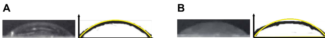
Figure 5.4: Characterization of mechanical stretches. Original CCD images (left) and the profiles (black curve in the right) of the deformed (A) PDMS membrane bonded on the pneumatic chamber and (B) nanofibrous membrane on the interstitial layer bonded on the pneumatic chamber under a theoretical strain of 15% (yellow curve).
