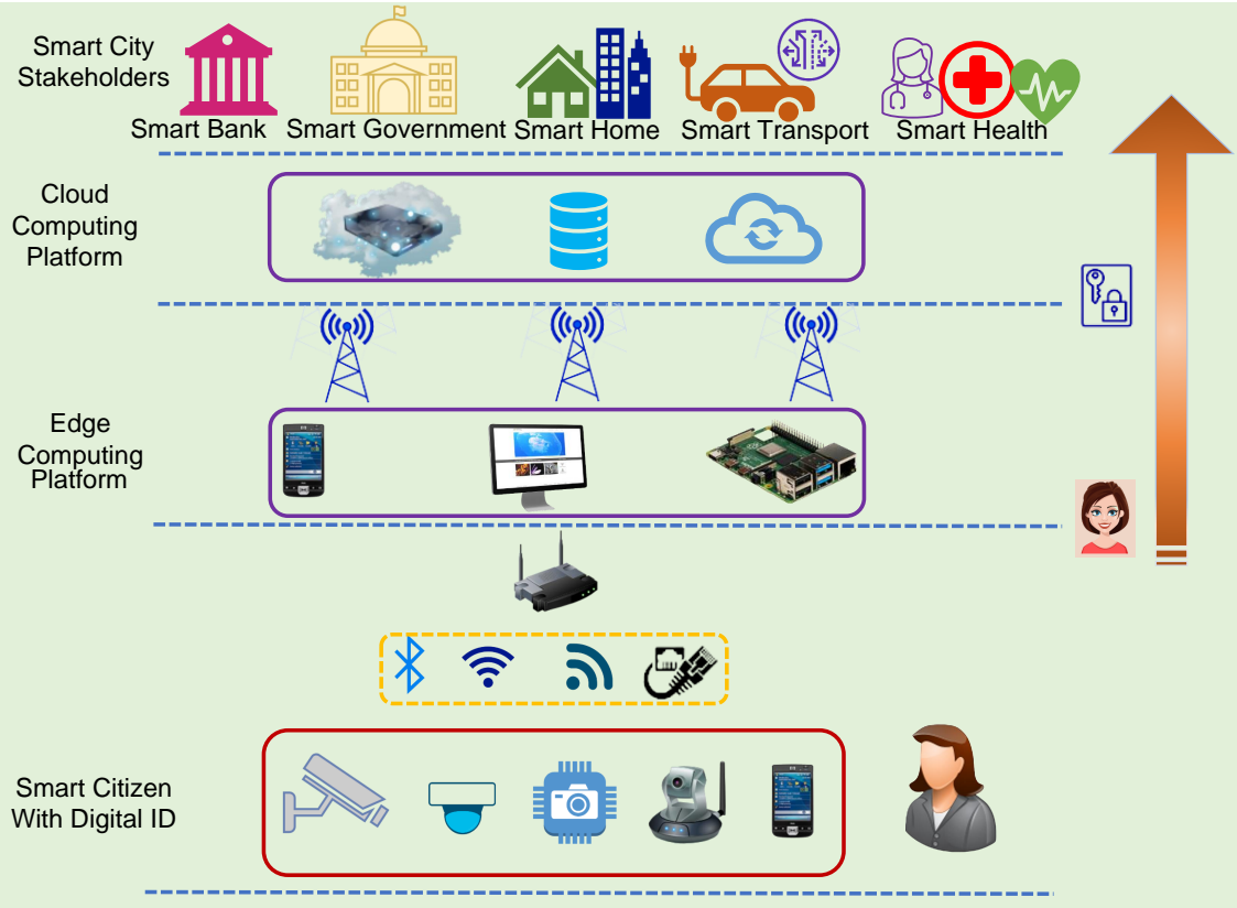
FIGURE 4.3. End-to-end system level framework for digital ID system in a smart city.
