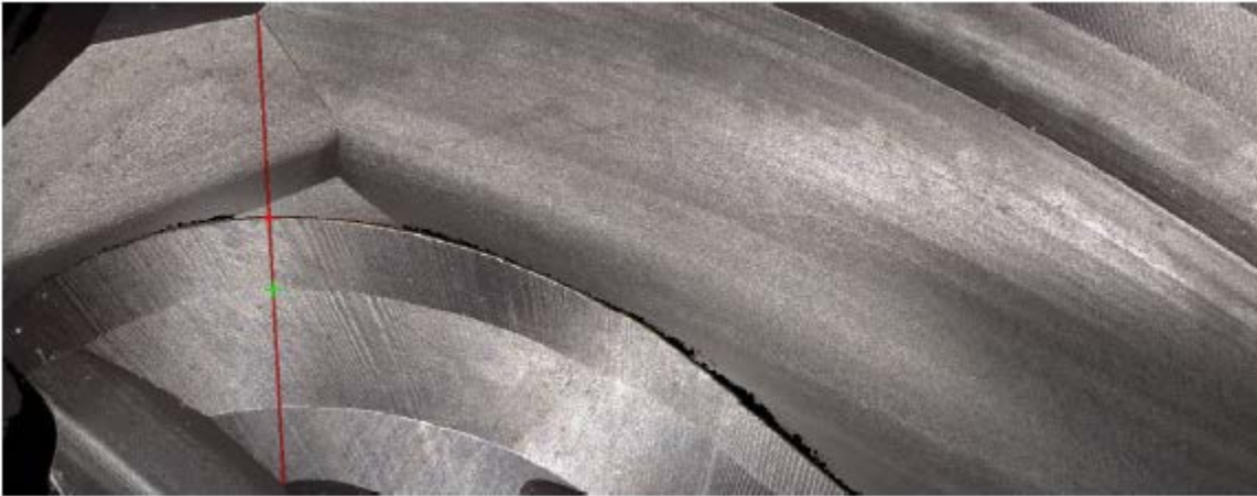
Figure 4.15: FVM scan of an unused ball-nose end mill with flank landing measurement in \mu\text{m} scale
