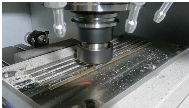
Figure 3.5: Ball-nose end milling of material deposited by DED Head
