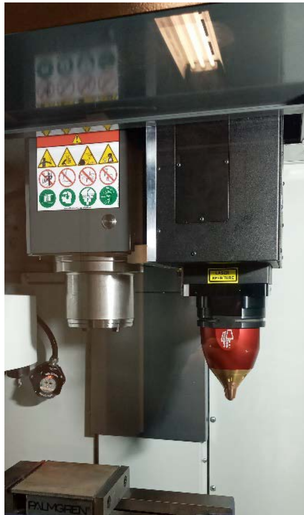
Figure 3.3: AHM inside work enclosure with original Spindle and adapted DED Head
