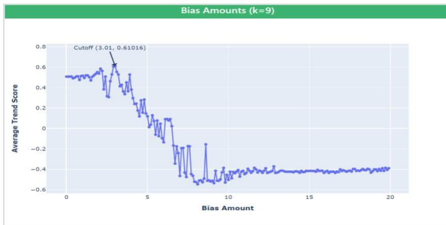
Figure 17 Line plot of average trend score per bias amount for k = 9 . A cutoff point is identified at a bias amount of 3.01 and an average trend score of 0.61.
