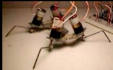
A Five Motor Advanced Walker (Still under experimentation)
