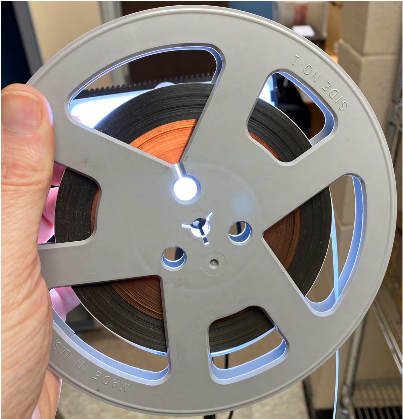
Figure 2 Acetate and polyester tape wound onto the same reel. The acetate is the translucent tape near the center.
