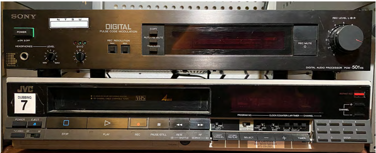
Figure 20 An F1 decoding setup with a PCM encoder and VHS player.
