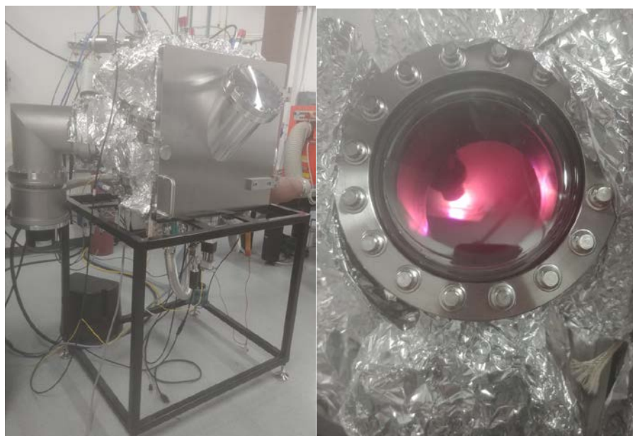
Figure 2.1: Sputtering box chamber (left) with magnetron sputtering in use (right).
