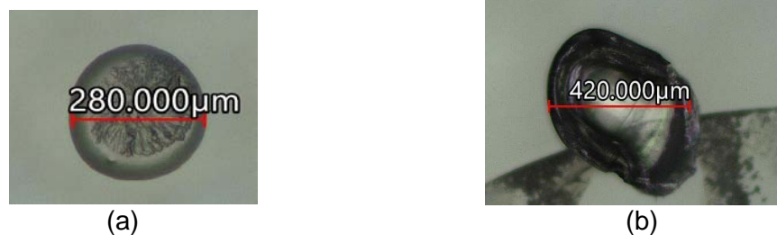
Figure 3-4: Image of micro spheroids obtained using laser optical microscope. (a) Micro spheroids with 420 microns diameter; (b) Micro spheroids with 280 microns diameter.
