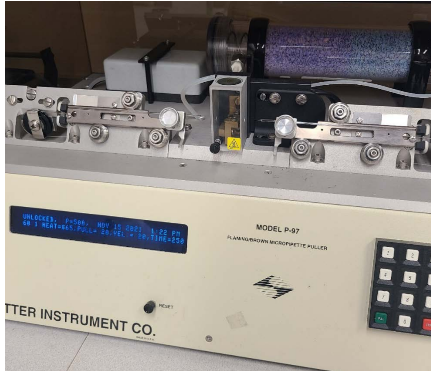
Figure 8: P-97 Pulling machine
