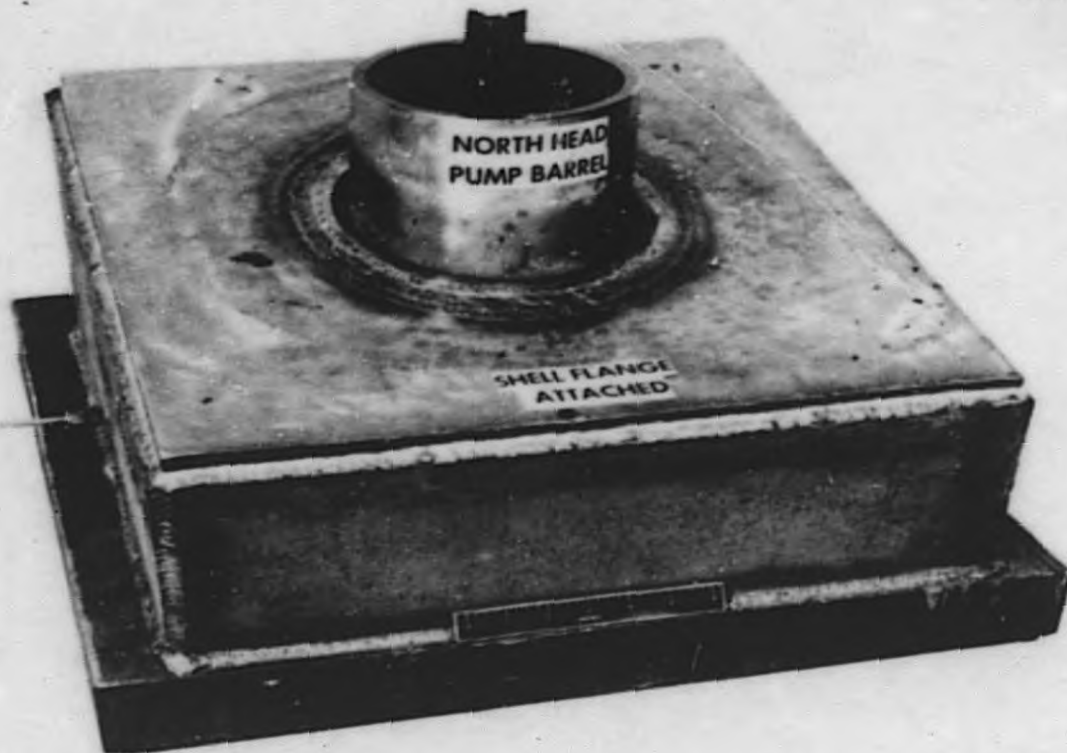
Fig. 3.4.10. Completed Test Weldment for Joining Pressure Shell Flange to Pump Barrel Sleeve.
