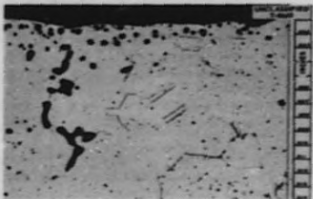
Fig. 3.1.2. Region of Maximum Attack in Inconel Forced-Circulation Loop 7425-41 Which Circulated the Fuel Mixture (No. 30) NaF-ZrF_4-UF_4 (50-46-4 mole %) for 1000 hr with a Maximum Wall Temperature of 1700^\circ F and a Maximum Fluid Temperature of 1650^\circ F . Etched with modified aqua regia. 250X. Reduced 32.5%. (Secret with caption)
