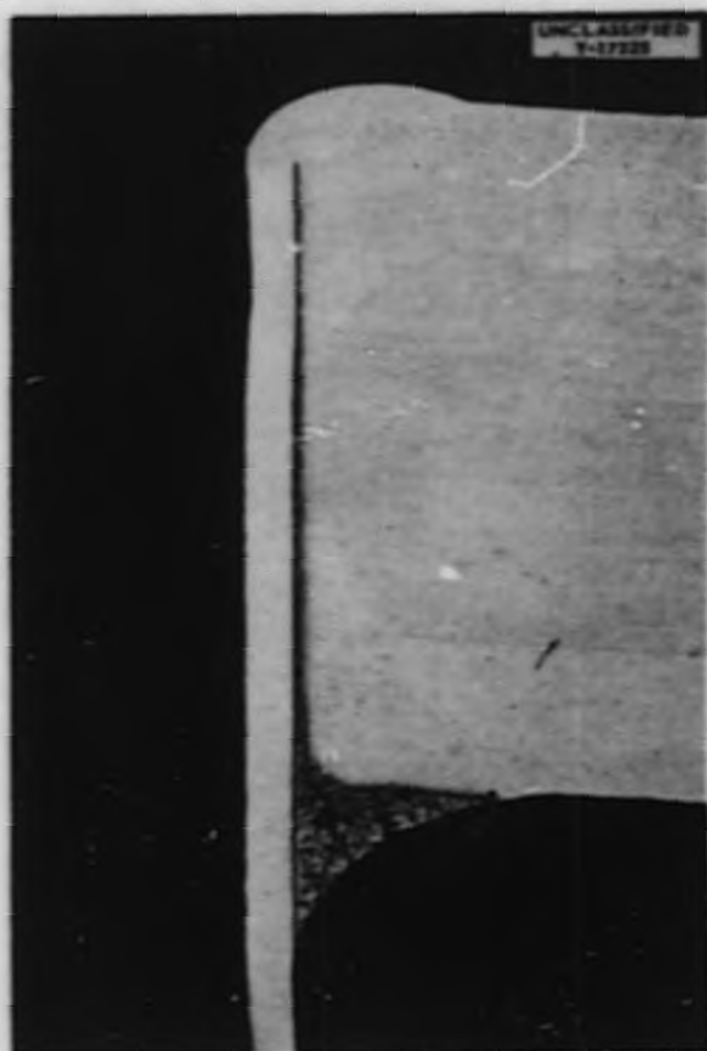
Fig. 3. Photomicrograph of a Typical Back-Brazed Tube-to-Header Weld. Etchant: oxalic acid. 12X. Reduced 14.5%.
