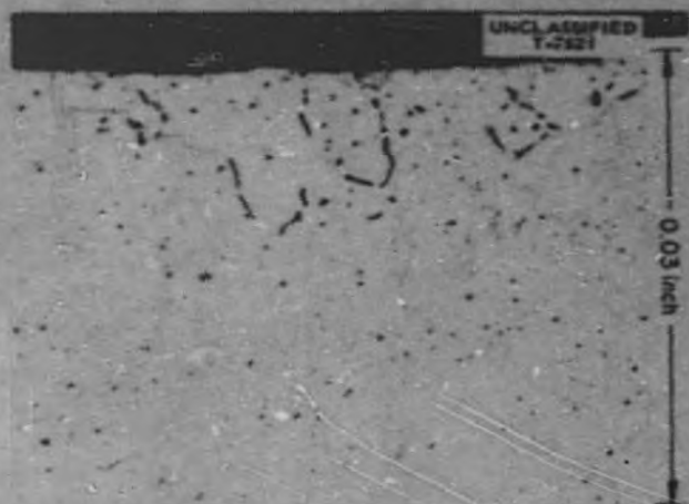
Fig. 5.1. Maximum Attack Found in Inconel Loop 4695-1 After Circulating NaF-ZrF 4 -(UF 4 + UF 3 ) (50-46-4 mole %, 2.2 wt % U as U 3+ ) for 385 hr at a Maximum Fluoride Mixture Temperature of 1500°F and a Reynolds Number of 10,000. 100X. Reduced 16%.
