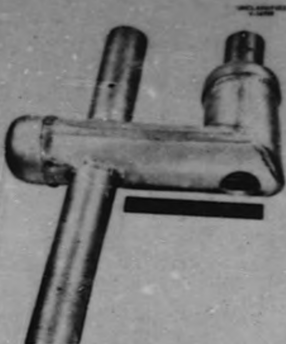
Fig. 6.8. Twenty-Tube Fuel-to-NaK Heat Exchanger Showing "Window" Cut in Pressure Shell to Permit Preplacement of Brazing Alloy on NaK Inlet End of the Tube Bundle.
