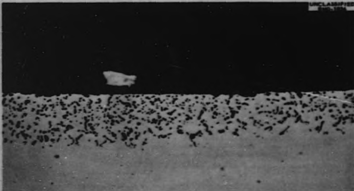
Fig. 41. Section Shown in Fig. 40 After Etching. 250X. (Secret with caption)
