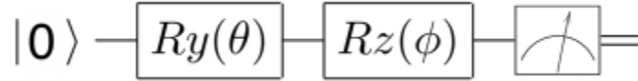
Figure 8.1: Mean-field circuit acting on a single qubit has been employed to determine the lowest bands of silicon. It consists of a polar rotation ( R_y ) followed by an azimuthal rotation ( R_z ). In last step, the expectation value of \hat{H}_k is measured.
