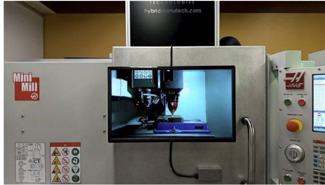
Figure 4: Hass Mini Mill equipped with a Hybrid Ambit Multi directed energy deposition system with Ytterbium laser from IPG, used for the manufacture of the test samples.
