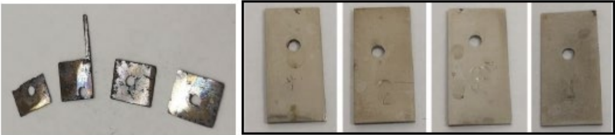
Figure 24: AM and control samples after 635 hours under corrosive atmosphere. AM presented different colorations with a shiny finish (left). Control presented a reddish and grayish finish (right).
