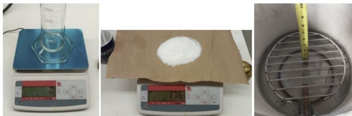
Figure 12: Measuring water (left) and salt (center) to prepare water- 3.5 wt.% NaCl solution for corrosion test. Verification of liquid level in autoclave during planned stop (right).
