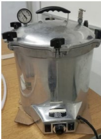
Figure 10: Autoclave used for the experiment. Model: All American 25X.
