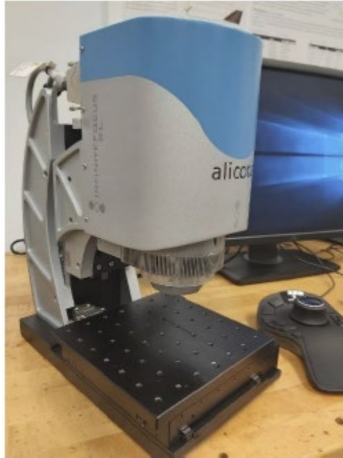
Figure 13: An Alicona InfiniteFocusSL optical 3D measurement system based on focus-variation microscopy, was used to obtain topographical information of the samples.
