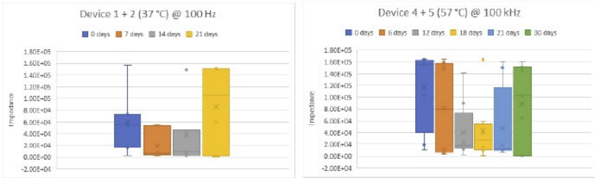
Figure 5.7: Box plot for electrode arrays 1+2 and electrodes 4+5 at 100 kHz
